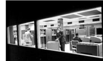
In **1960** an **IBM 7090** was used to perform design and development calculations for the Saturn rocket project. The IBM 7090 provided data from storage in 2.18 millionths of a second and added 13,740,000 figures a minute.
