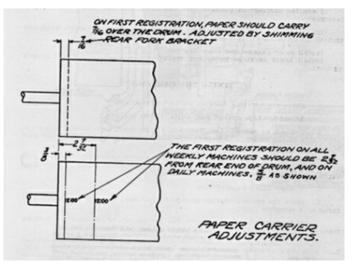
the first figure on a weekly dial and on a daily or double drum, the distance will be 3/8".
