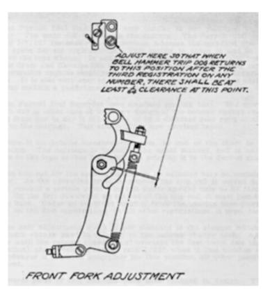
10. Adjust the lift rod for the automatic locking pawl for 1/64" clearance between the locking pawl and abutment.
