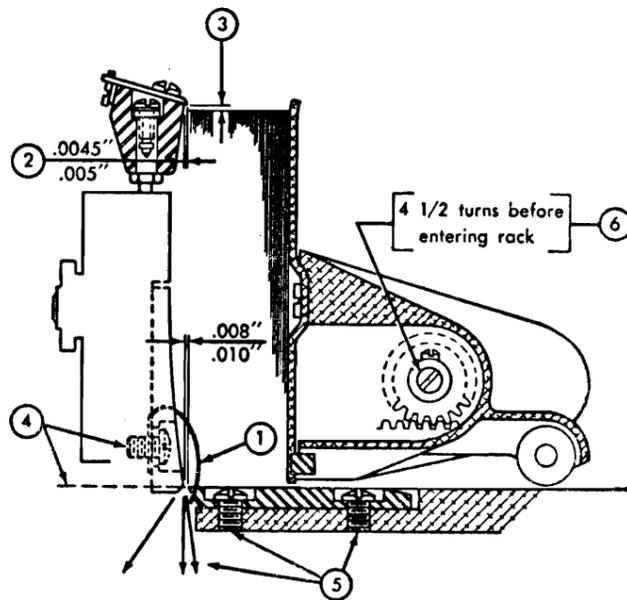
Figure 19. Card Feed Unit Adjustment
