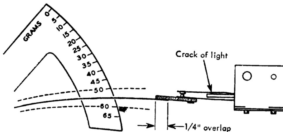
Figure 26. Interposer Bail Contact Adjustment
