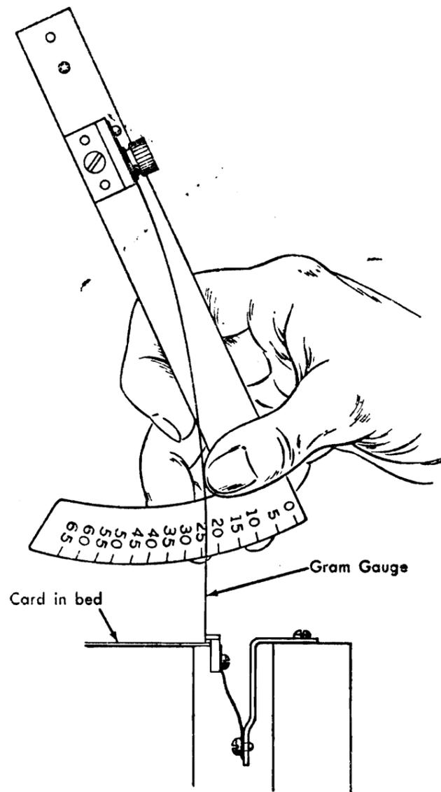
Figure 8. Pressure Rail Adjustment
