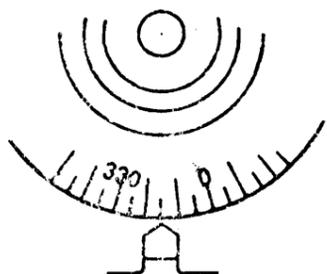
Figure 22. Armature Clearance Adjustment
