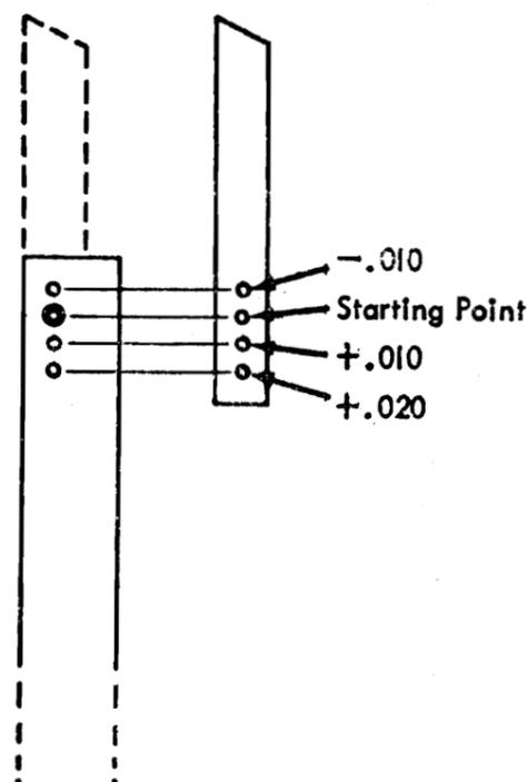
Figure 35. Adjustable Penetration - Type 26
