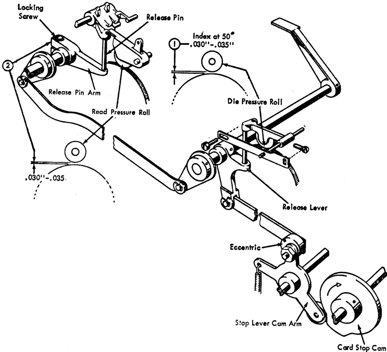
Figure 3. Pressure Roll Adjustments
