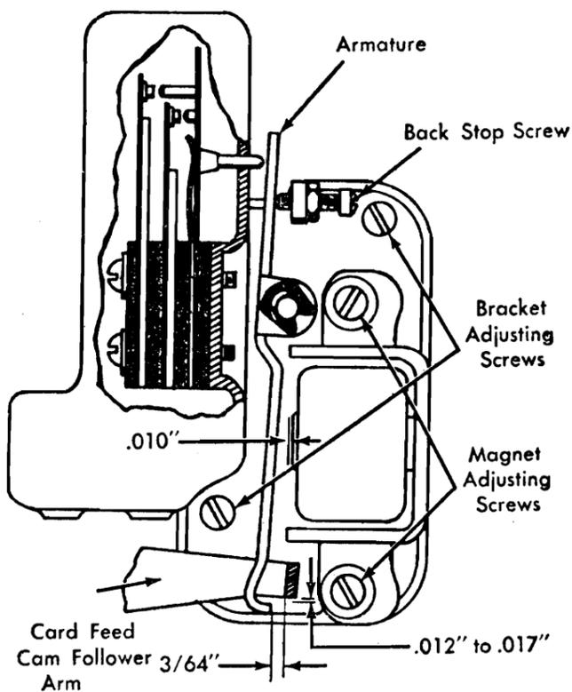
Figure 18. Latch Magnet Adjustment
