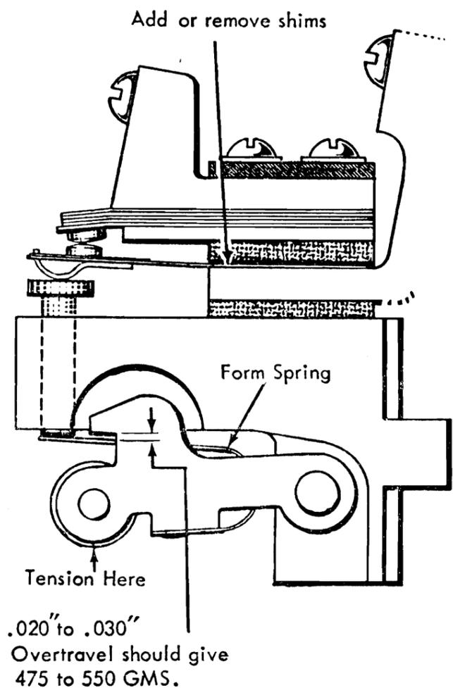
Figure 27. Circuit Breaker Adjustment
