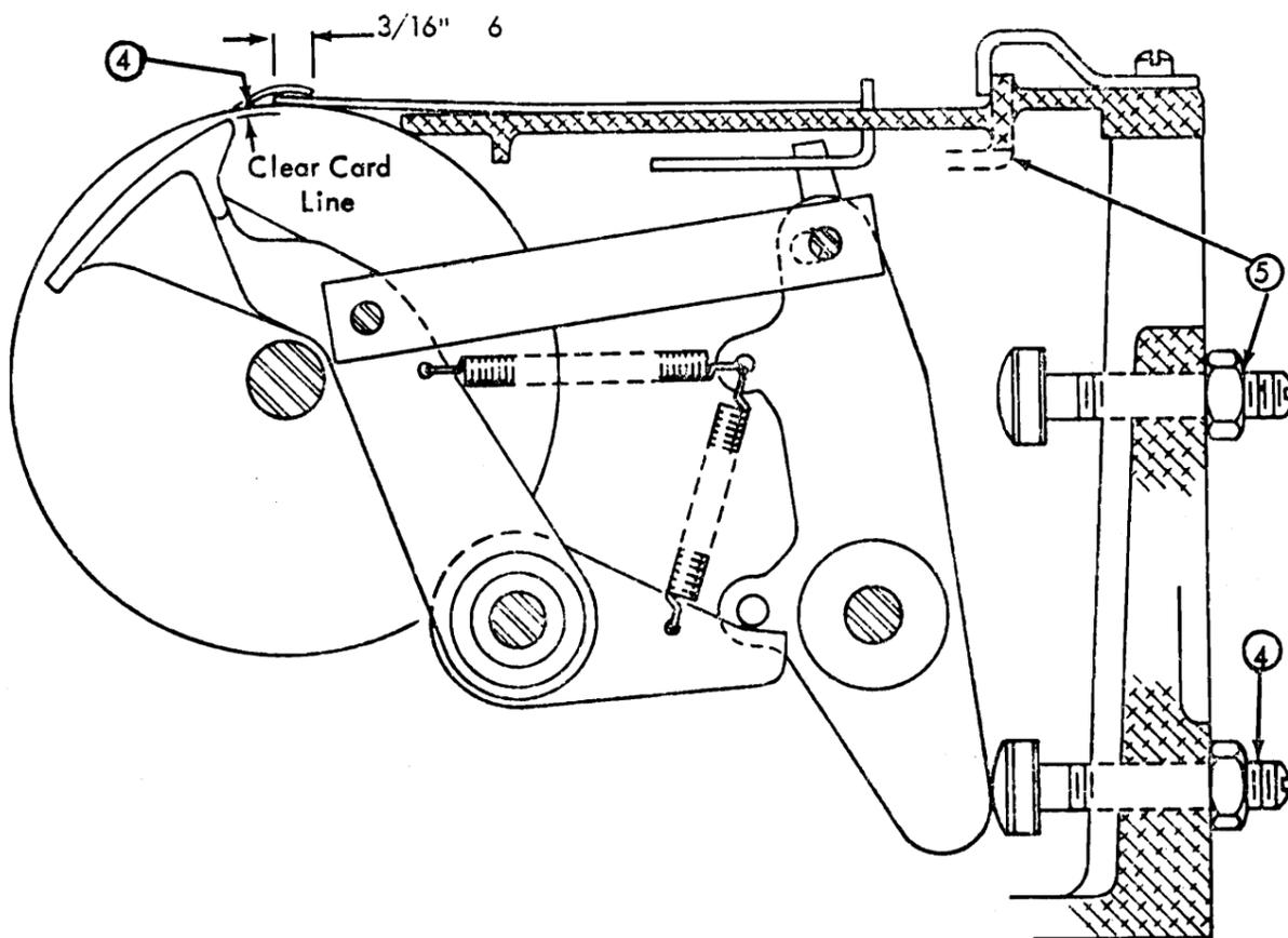
Figure 11. Stacker Adjustment
