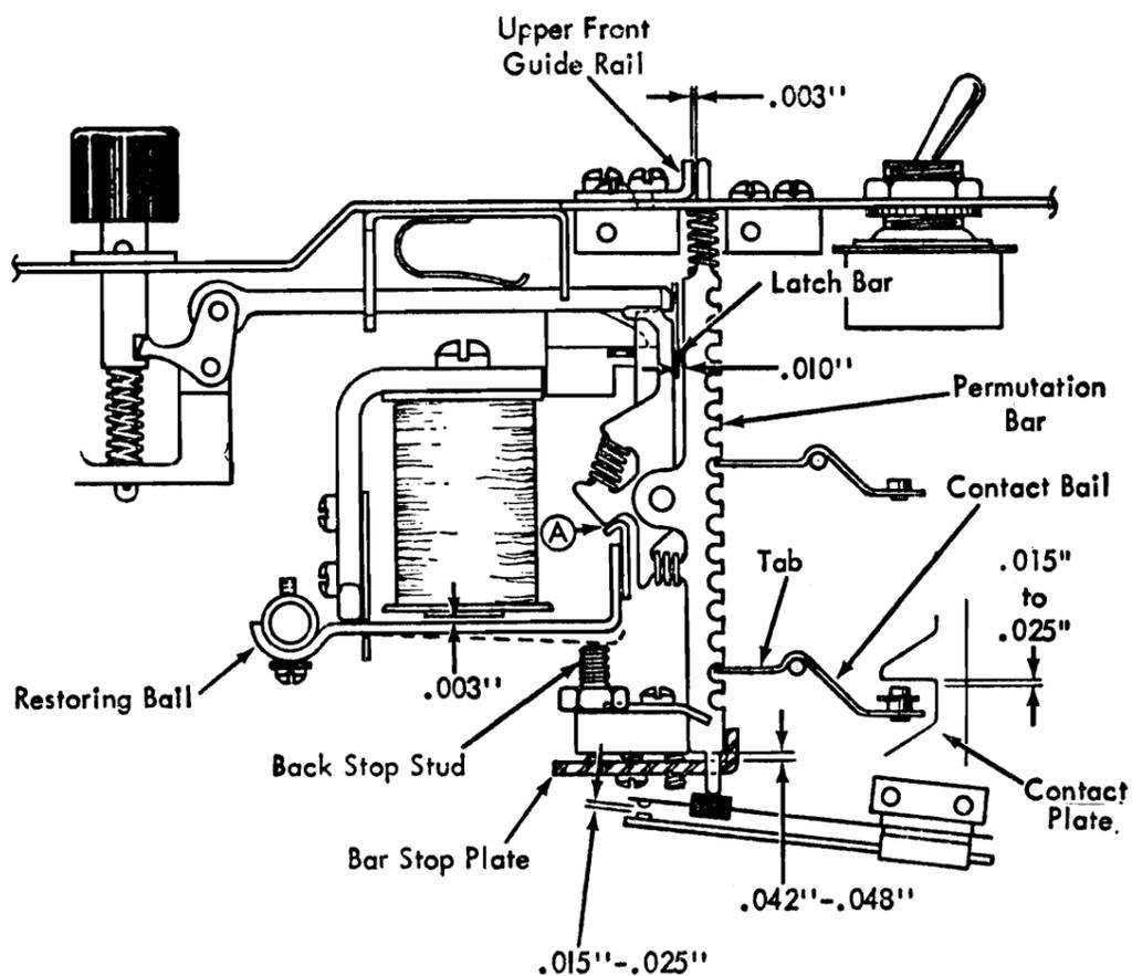
Figure 29. Keyboard Adjustment
