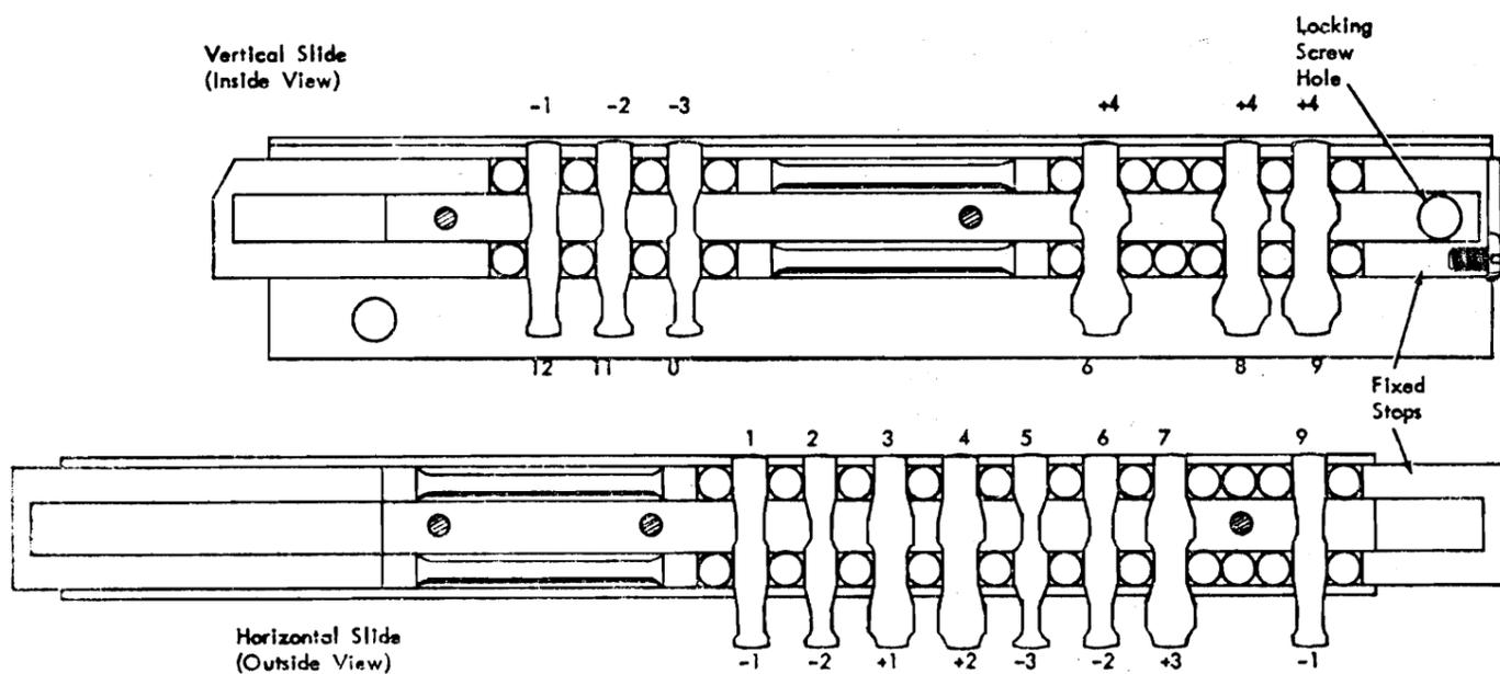
Figure 33. Print Interposer Assembly
