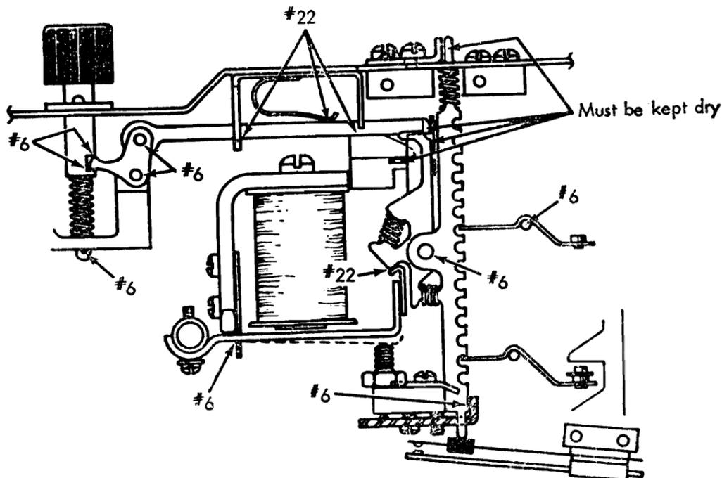
Figure 30. Keyboard Lubrication
