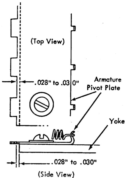
Figure 24. Armature Pivot Adjustment
