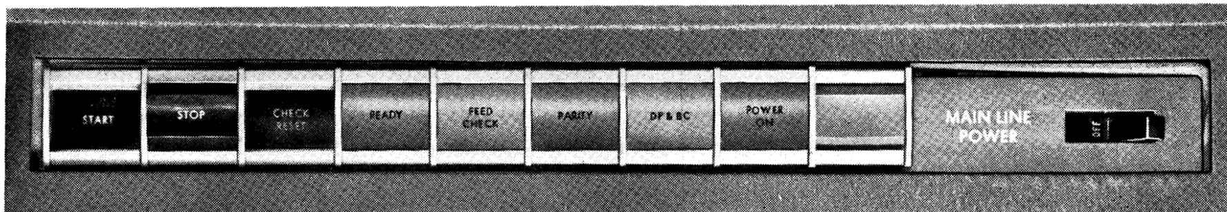
FIGURE 89. 323 PUNCH OPERATING KEYS AND LIGHTS
