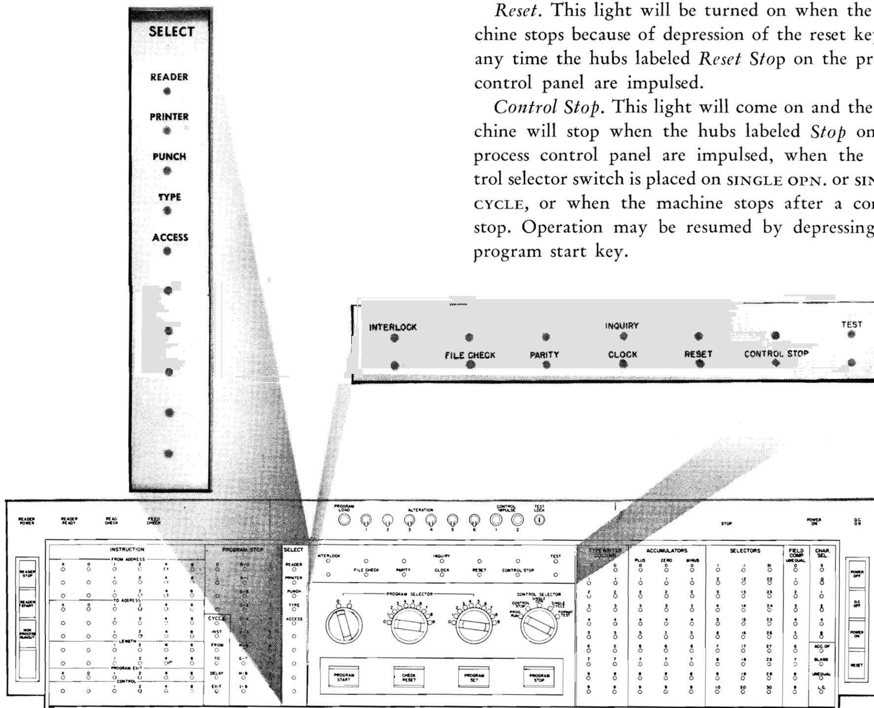
FIGURE 55. ERROR INDICATION AND CONTROL LIGHTS
