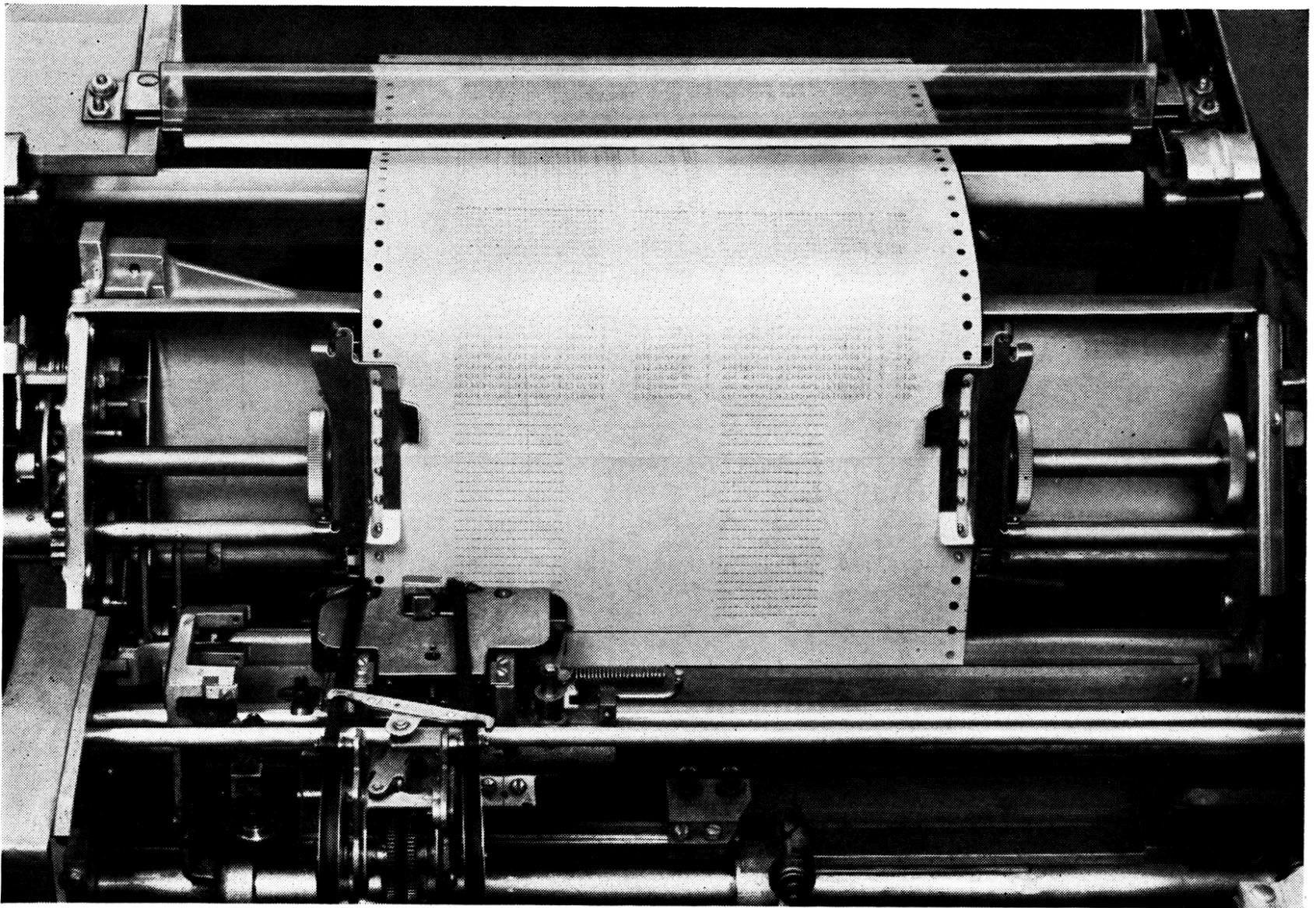
FIGURE 74. TAPE-CONTROLLED CARRIAGE
