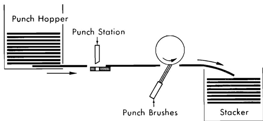
FIGURE 88. PUNCH FEED SCHEMATIC
