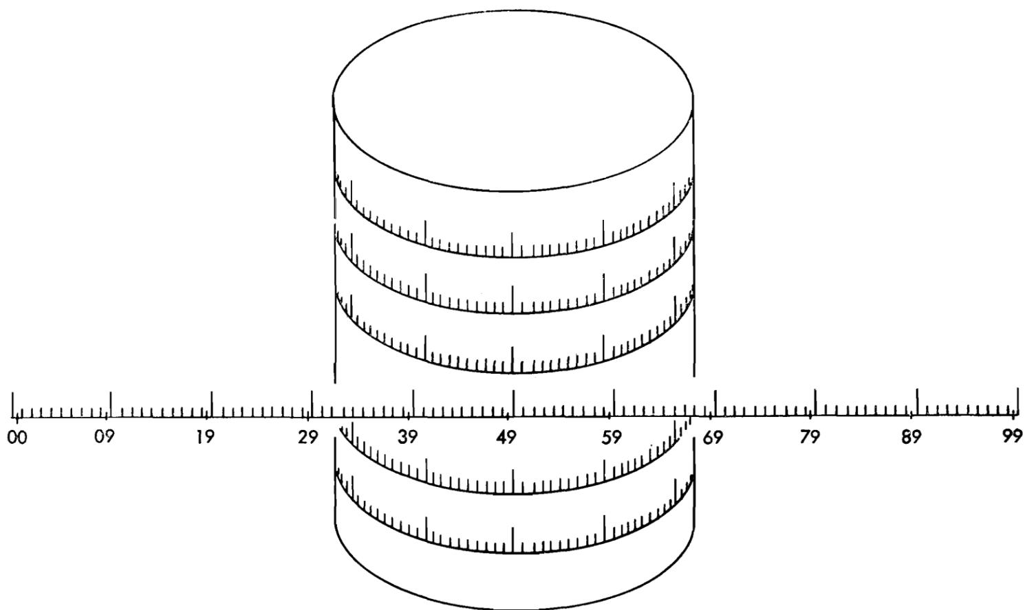
FIGURE 7. GRAPHIC REPRESENTATION OF DRUM TRACKS AND DISK TRACKS
