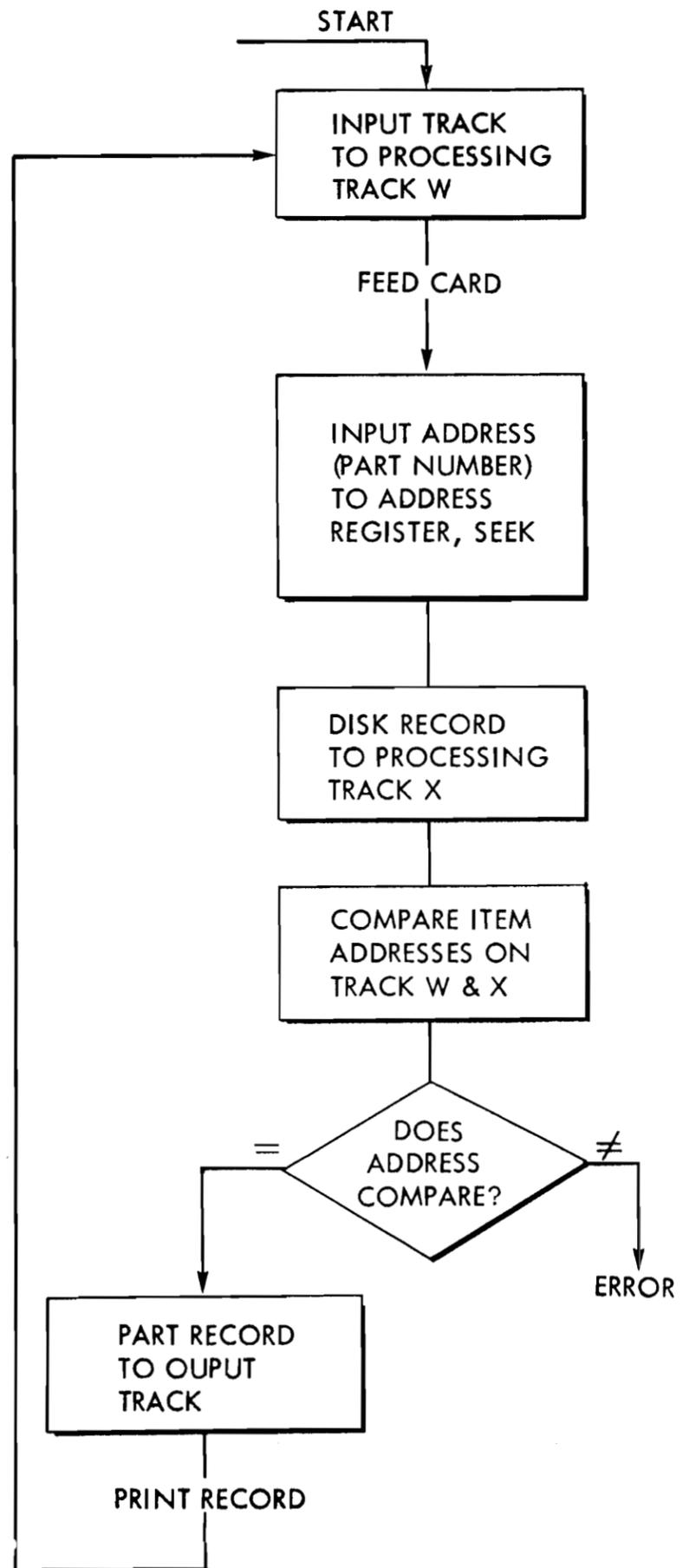
FIGURE 22. BLOCK DIAGRAM OF A DISK STORAGE-UNLOADING PROGRAM
