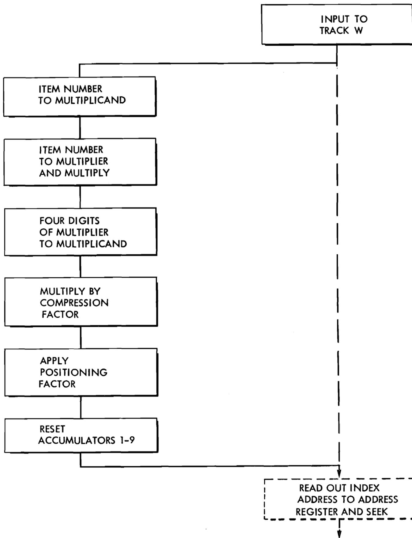
FIGURE 40. BLOCK DIAGRAM — GENERATING THE INDEX ADDRESS
