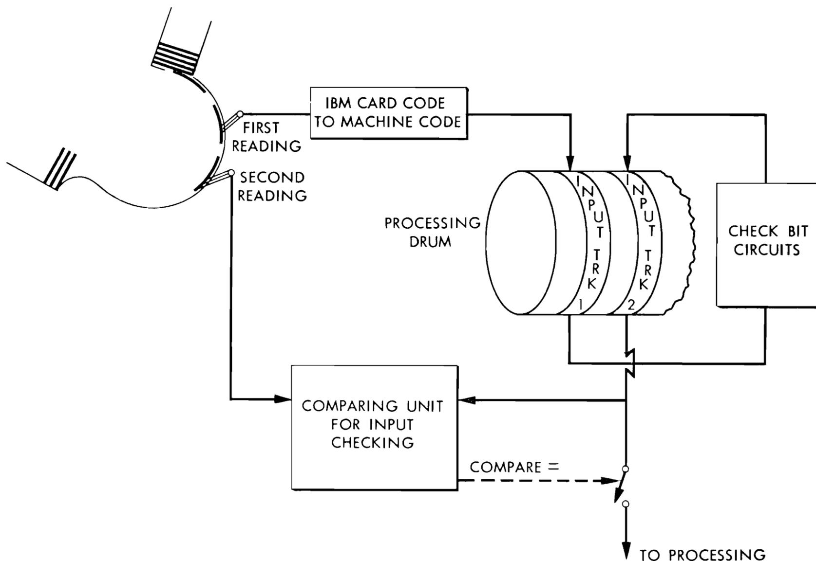
FIGURE 45. CHECKING OF INPUT CARD READING
