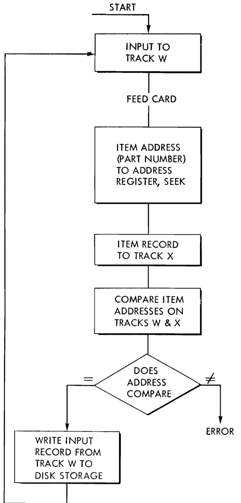
FIGURE 20. BLOCK DIAGRAM OF A DISK STORAGE LOADING PROGRAM
