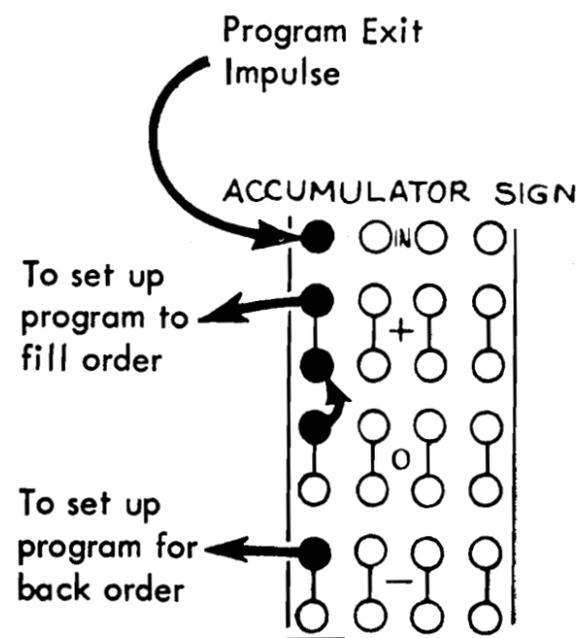
FIGURE 6. METHOD OF BRANCHING BY CONTROL PANEL WIRING
