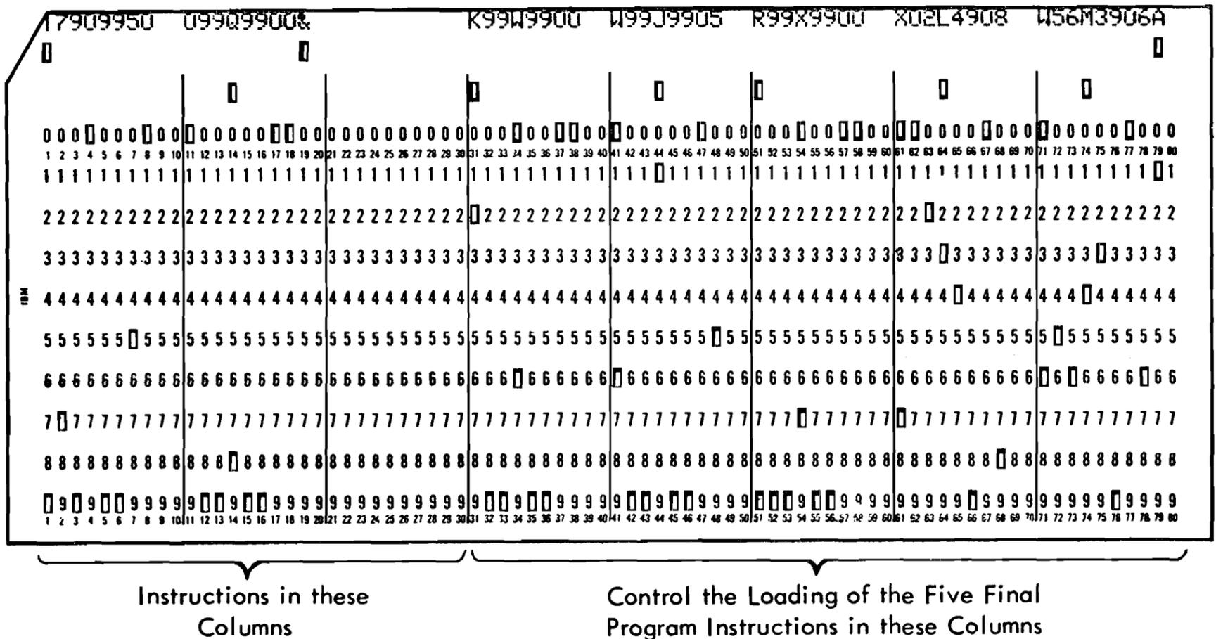
FIGURE 12. CARD USED FOR PROGRAM LOADING
