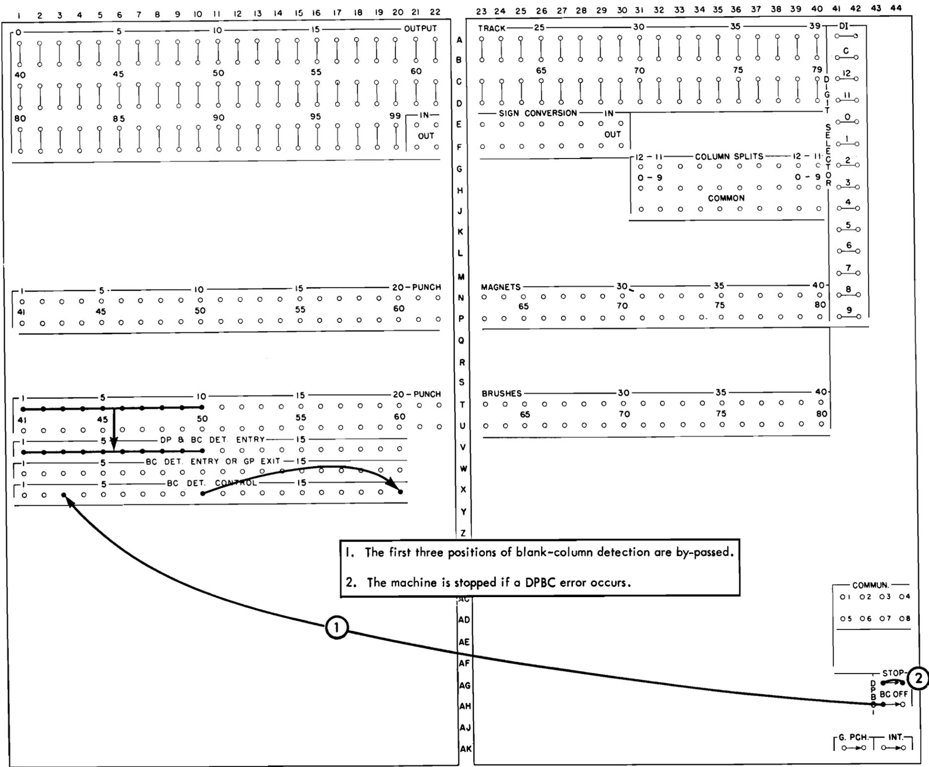
FIGURE 96. DOUBLE-PUNCH AND BLANK-COLUMN DETECTION
