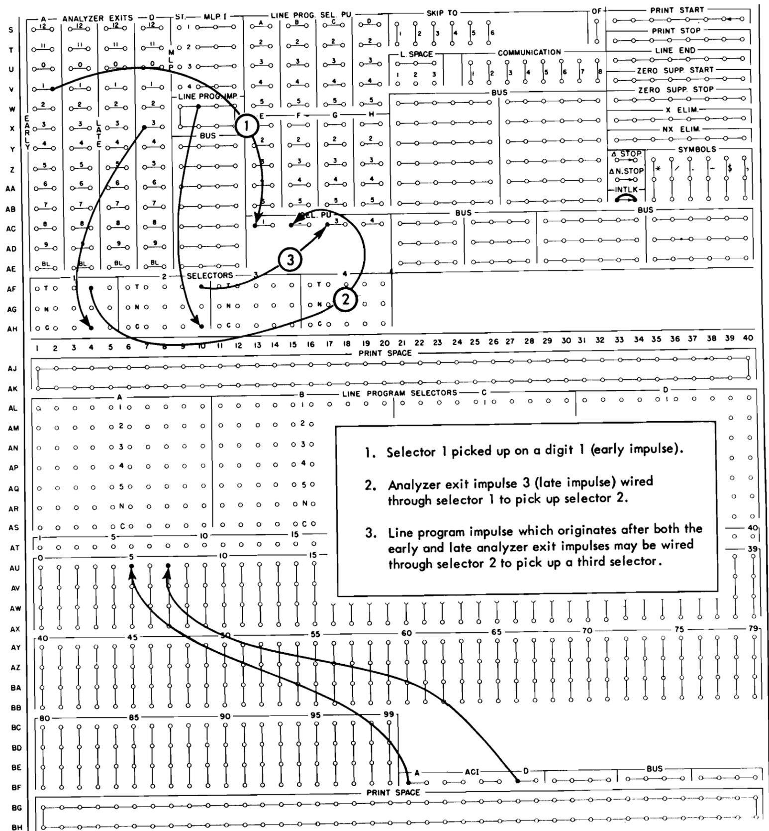
FIGURE 85. SERIES WIRING TO ILLUSTRATE TIMINGS
