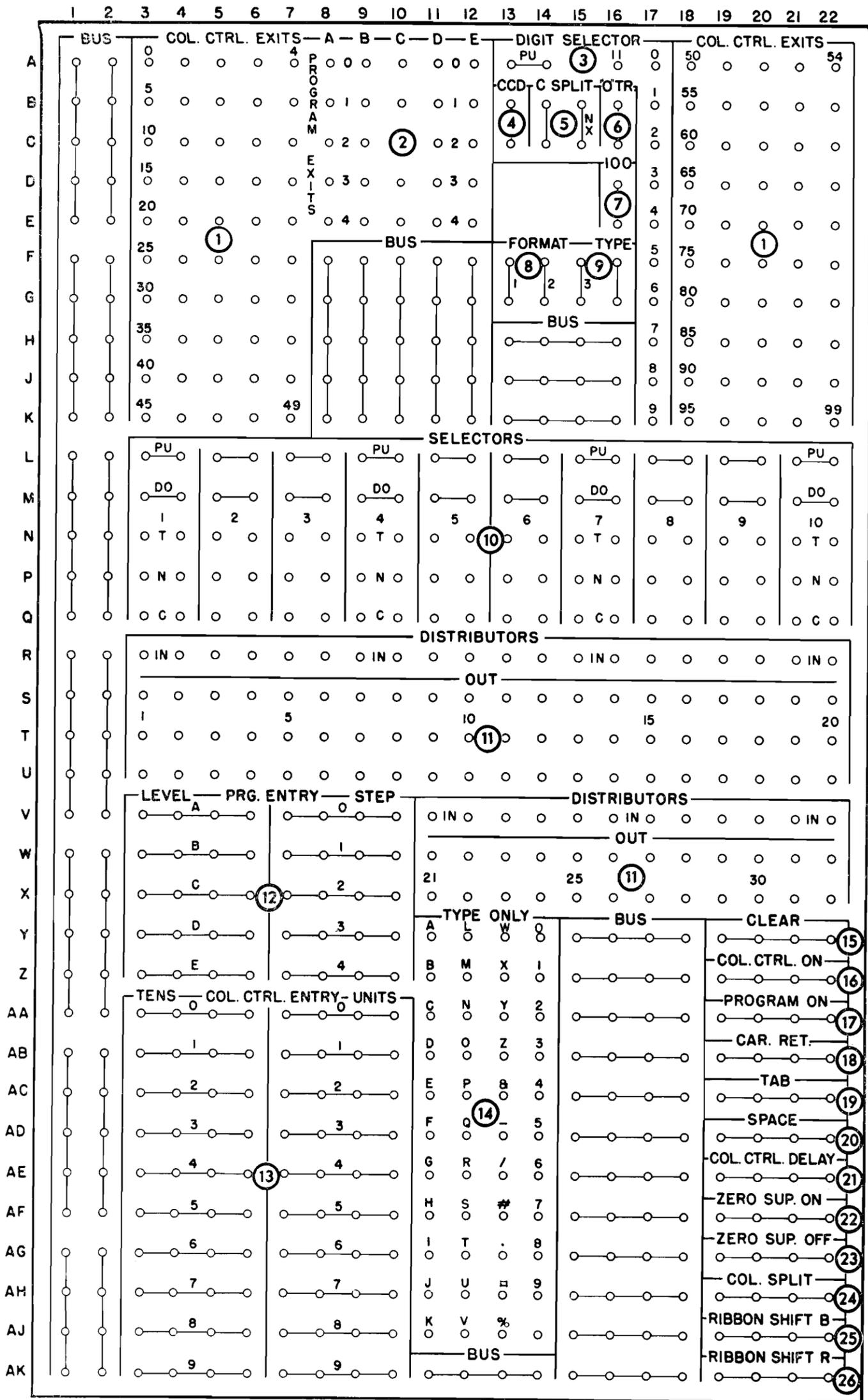
FIGURE 101. 380 TYPEWRITER CONTROL PANEL
