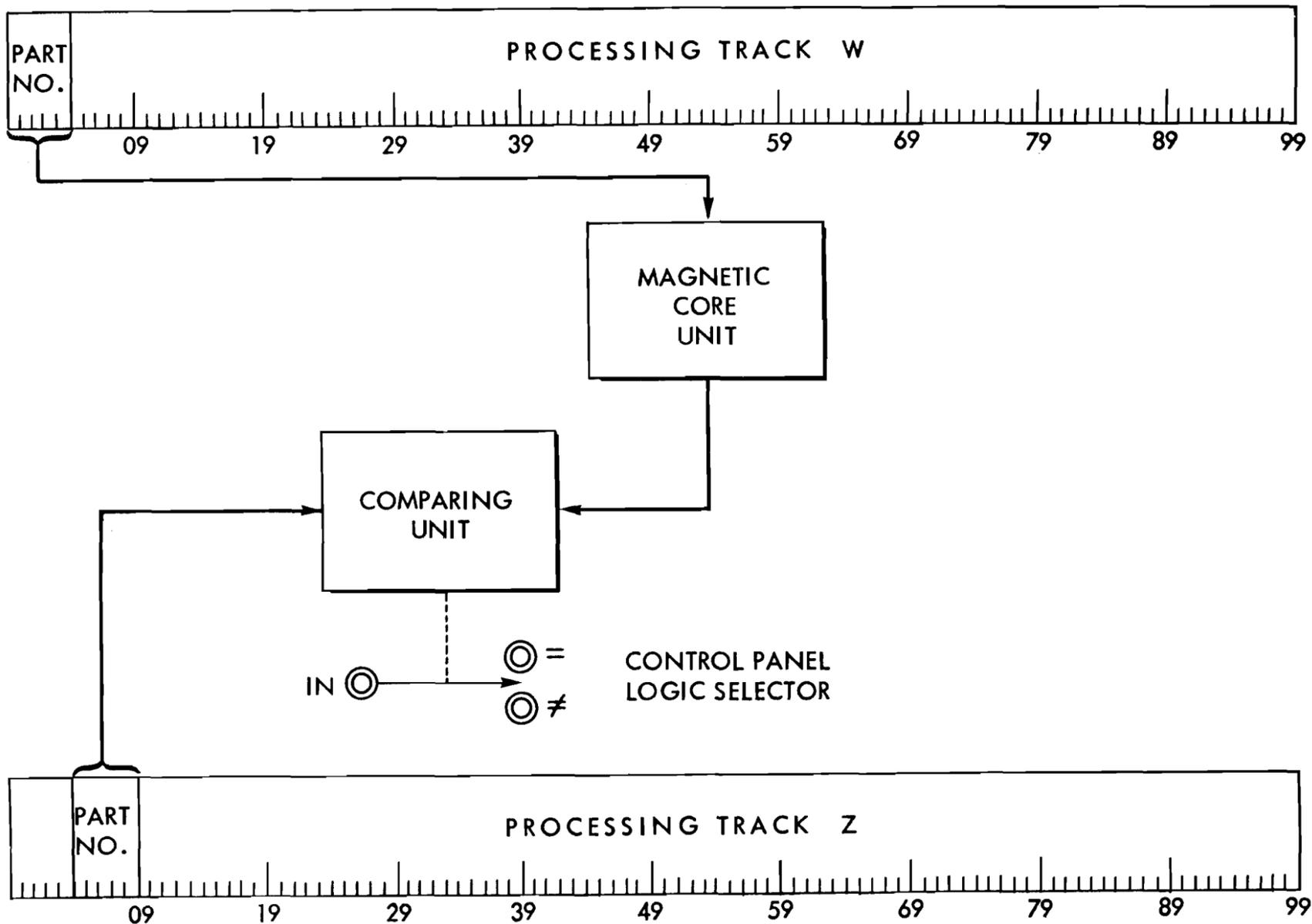
FIGURE 16. SCHEMATIC OF A COMPARING OPERATION
