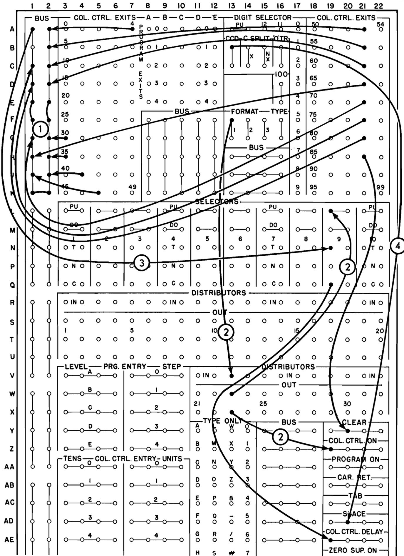
Wiring necessary to print the following disk record inserting one space between each column.
