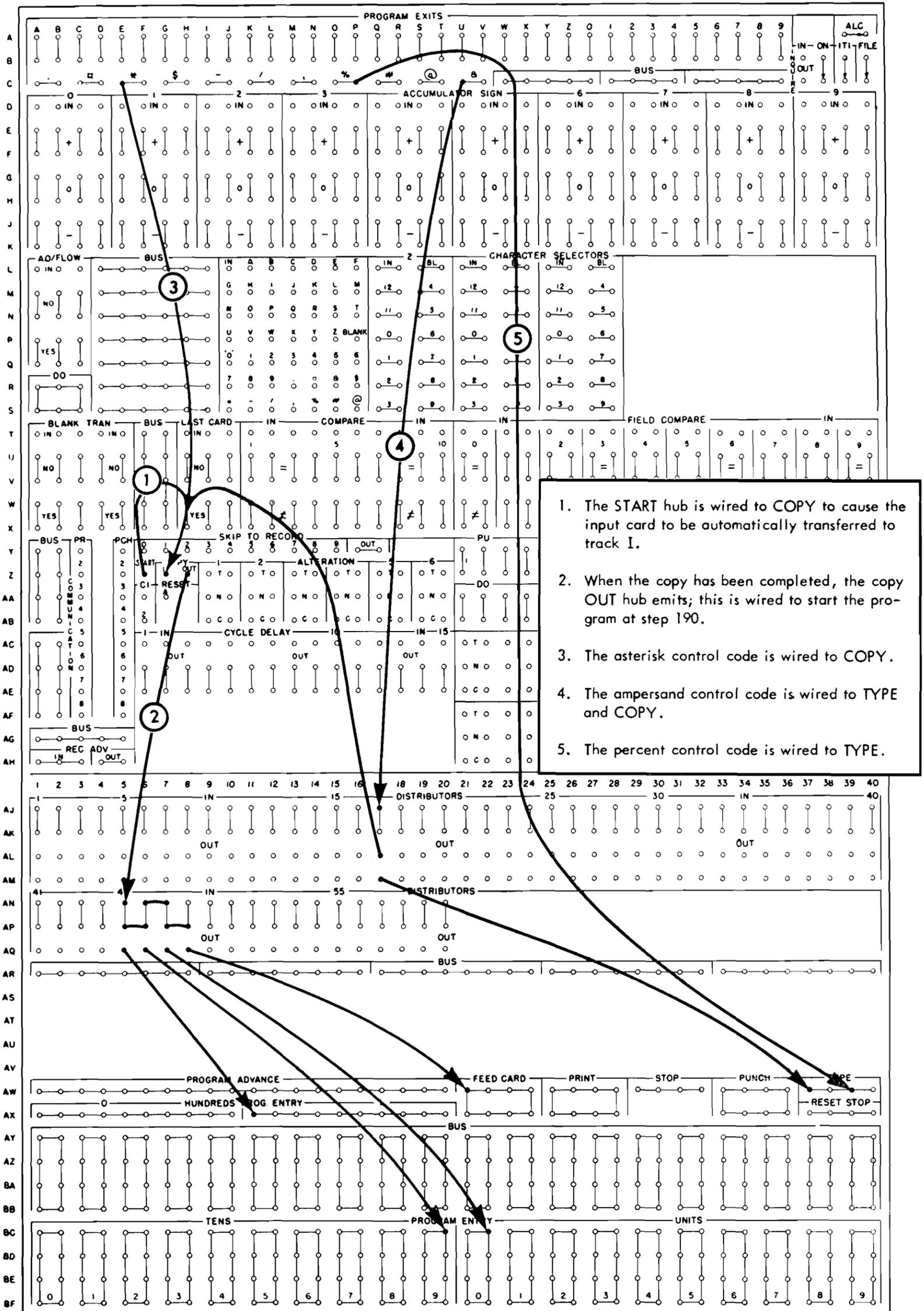
1. The START hub is wired to COPY to cause the input card to be automatically transferred to track I.
