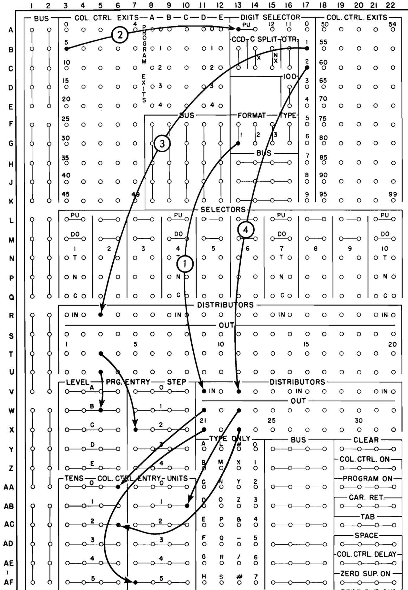
FIGURE 62. ALTERATION OF FORMAT CONTROL
