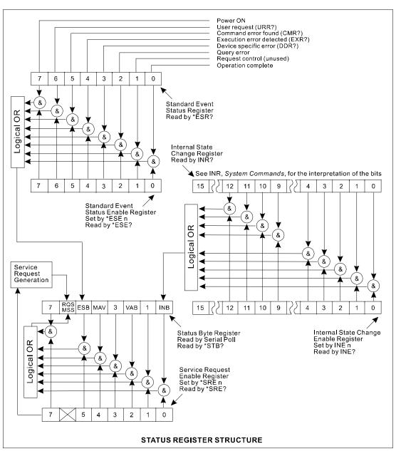
The register structure contains one more register, not shown in the above figure. This is the Parallel Poll Enable Register (PRE), which acts exactly like the Service Request Enable Register (SRE), but sets the "ist" bit (also not shown in the figure), used in the Parallel Poll. The "ist" bit can also be read with the "\*IST?" query.
