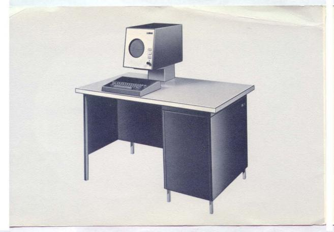
The IBM 1015 INQUIRY DISPLAY TERMINAL provides fast, flexible, remote inquiry capabilities where documentation is not desired at the inquiry location.
