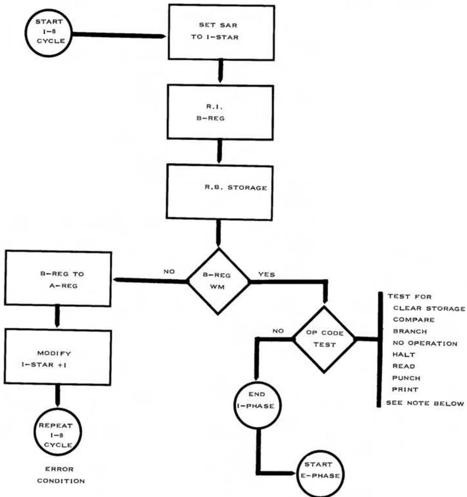
NOTE - THE OP CODE IS TESTED TO DETERMINE IF THE INSTRUCTION REQUIRES SOME SET-UP OPERATIONS TO BE PERFORMED BEFORE ENDING I-PHASE. THE DIAGRAMS FOR THE SPECIFIC INSTRUCTIONS LISTED INCLUDE THE APPROPRIATE SET-UP OPERATIONS.
