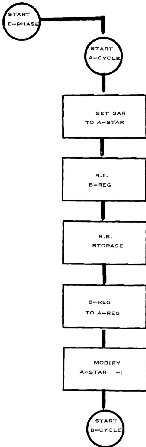
THIS TYPE OF A-CYCLE IS COMMON TO MANY 1401 INSTRUCTIONS. IT WILL NOT BE REPEATED FOR EACH ONE BUT REFERENCE WILL BE MADE TO THIS PAGE FOR THE MOVE, MOVE DIGIT, MOVE ZONE, LOAD, COMPARE, MOVE AND ZERO SUPPRESS, EDIT, RESET ADD, RESET SUBTRACT, TRUE ADD, AND COMPLEMENT ADD INSTRUCTIONS.
