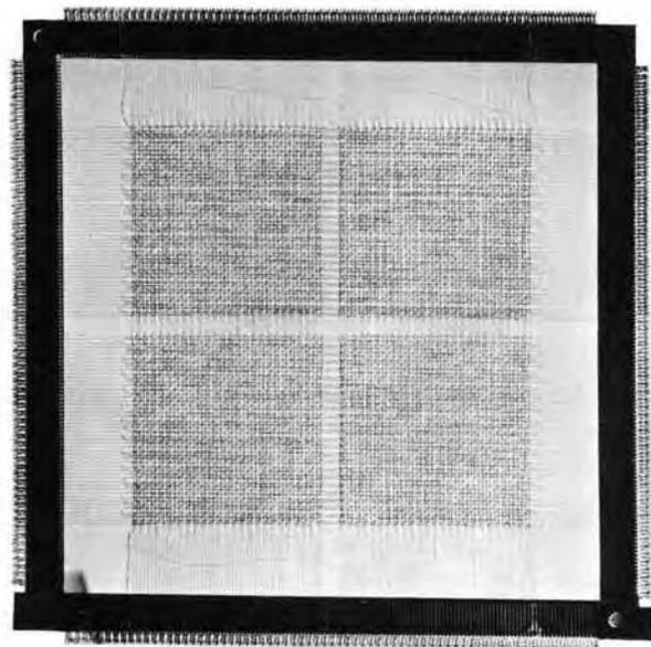
Figure 9. Magnetic Core Storage Unit
