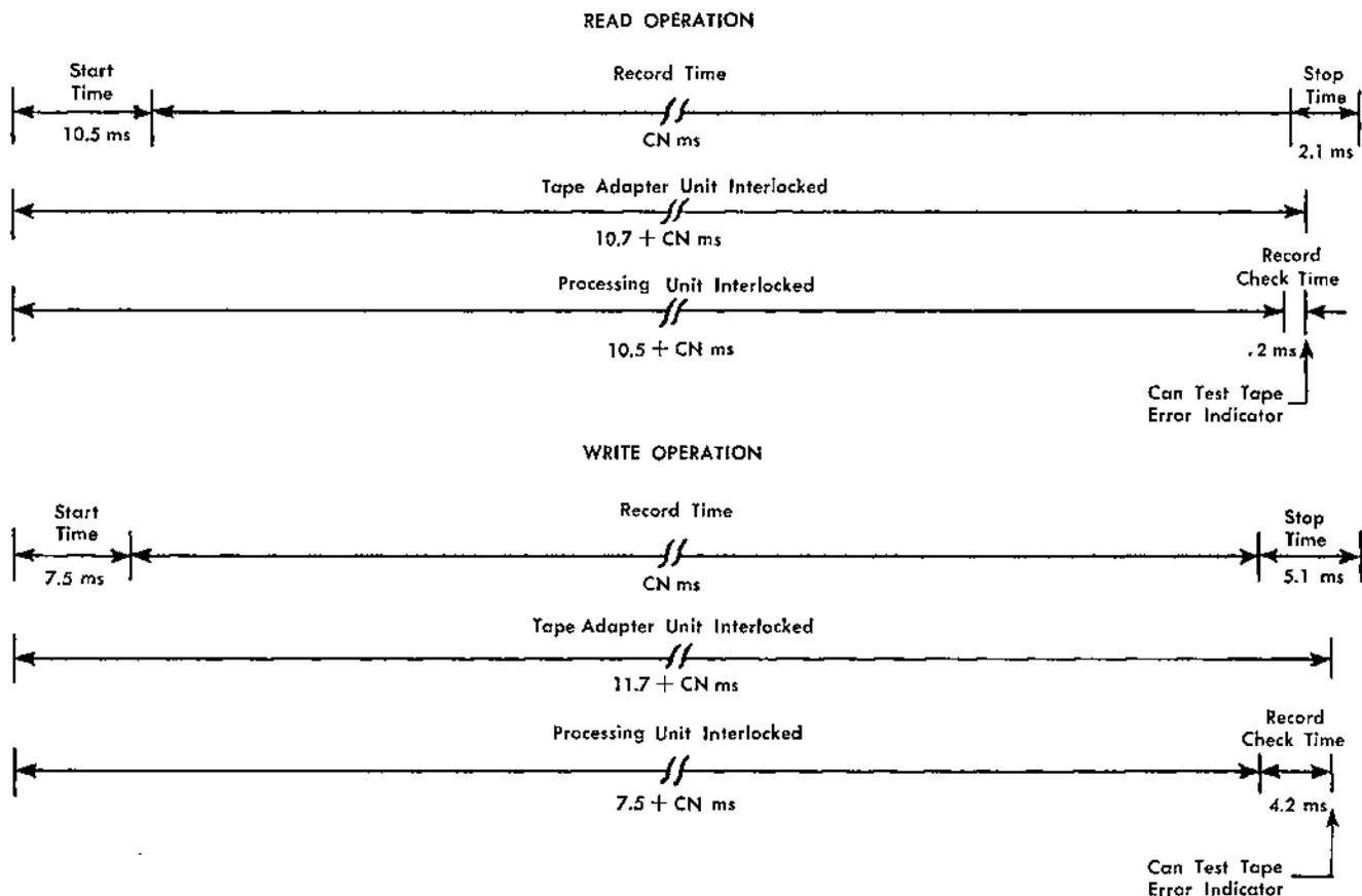
Figure 245. IBM 729, Model II, Read-Write Tape Timing
