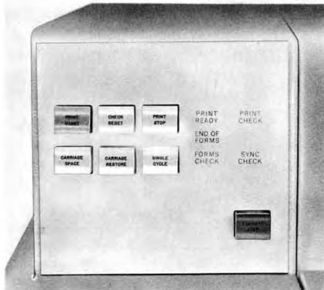
Figure 198. IBM 1403 Printer Operating Keys and Lights
