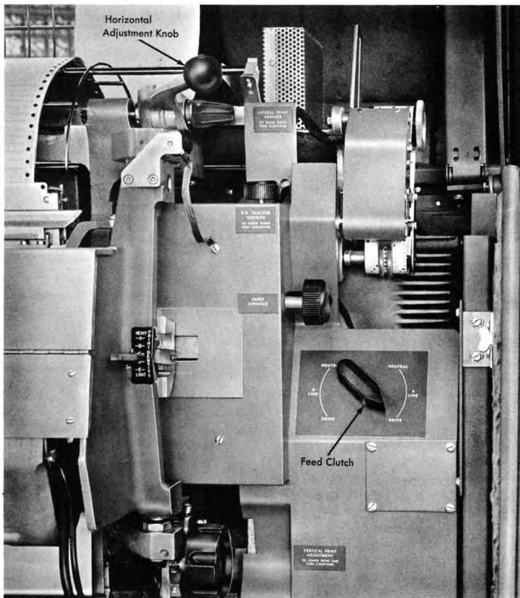
Figure 200. Manual Controls
