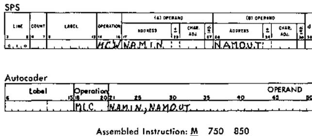
Figure 50. Move (Two-Address)
