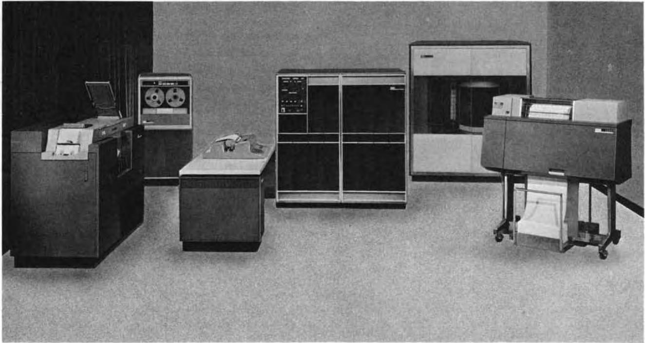
Figure 1. IBM RAMAC 1401 Data Processing System
