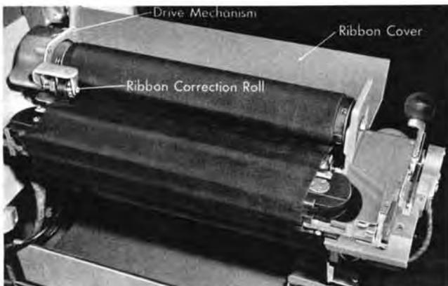
Figure 208. Ribbon Mechanism
