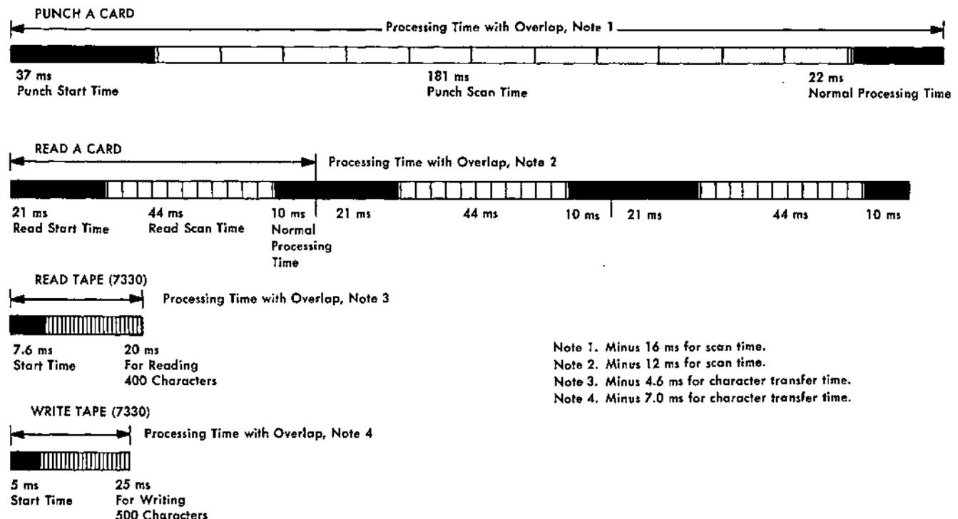
Figure 250. Comparison of Standard and Overlapped Processing Times
