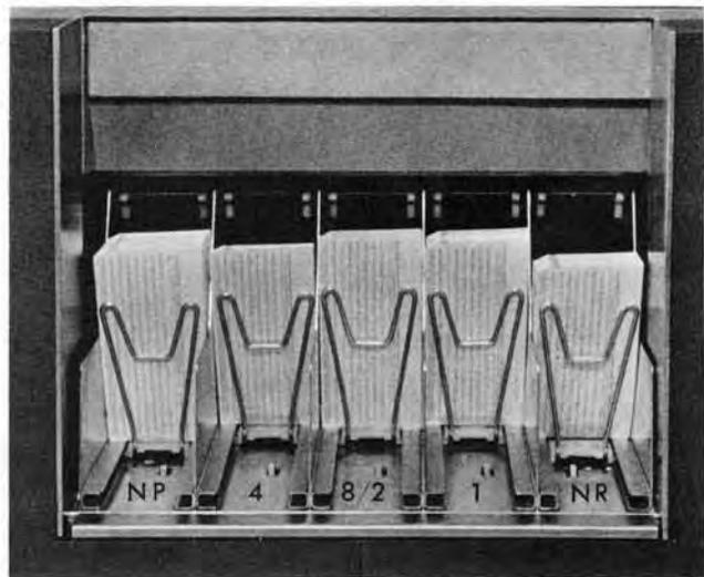
Figure 6. Radial Stackers
