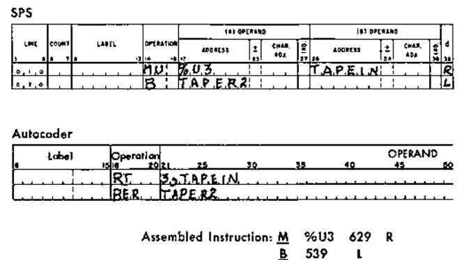
Figure 108. Test for Transmission Error
