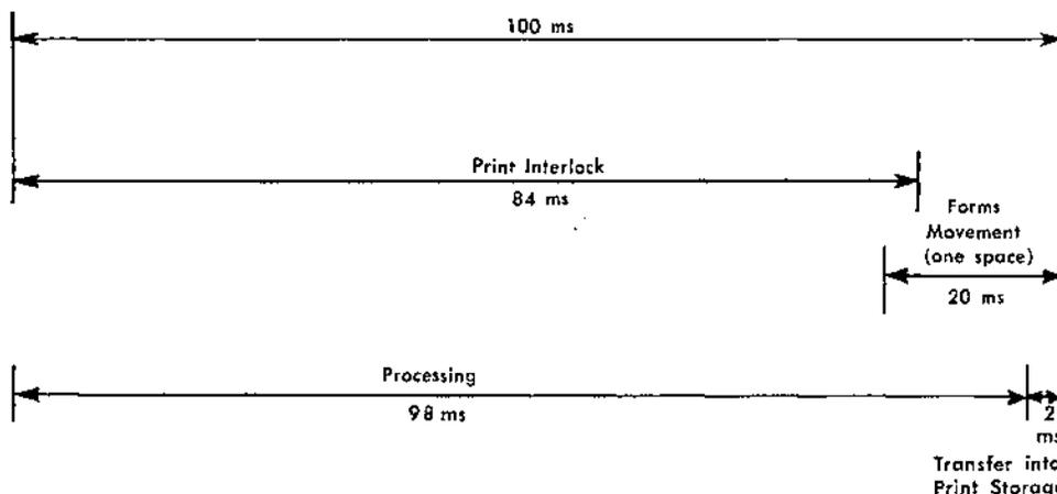
Figure 229. Print Timing Chart (with Print Storage)
