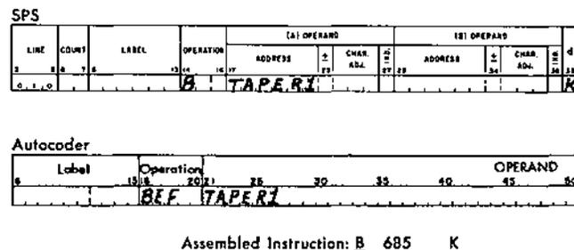
Figure 107. Test for End of Reel
