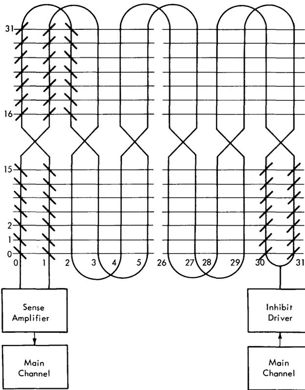
Figure 2-10. Sense/Inhibit Line
