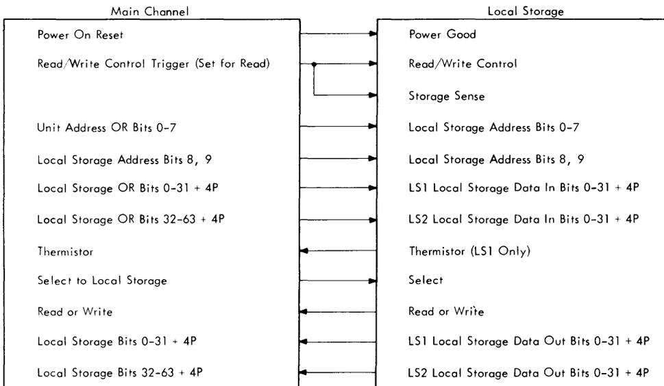
Figure 2-31. Local Storage to Main Channel Interface
