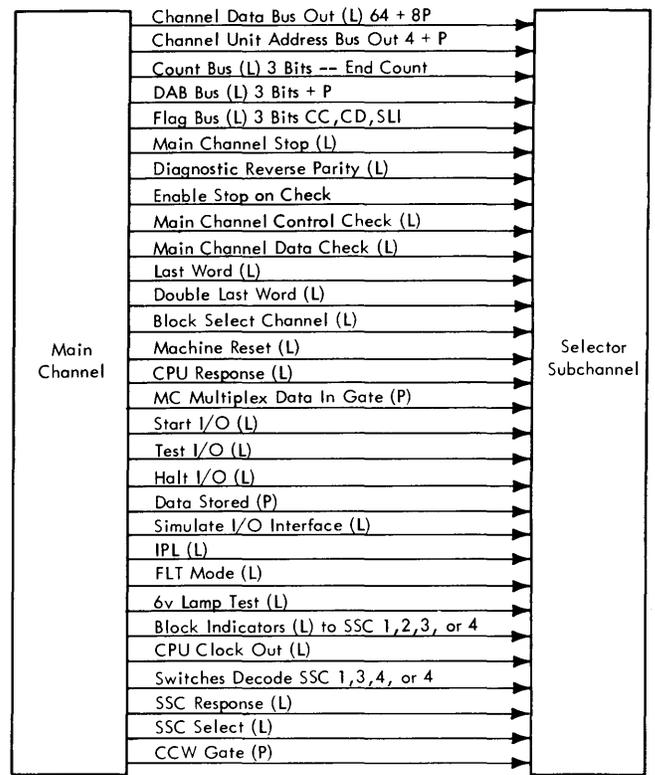
Figure 2-30. Main Channel to Selector Subchannel Interface
