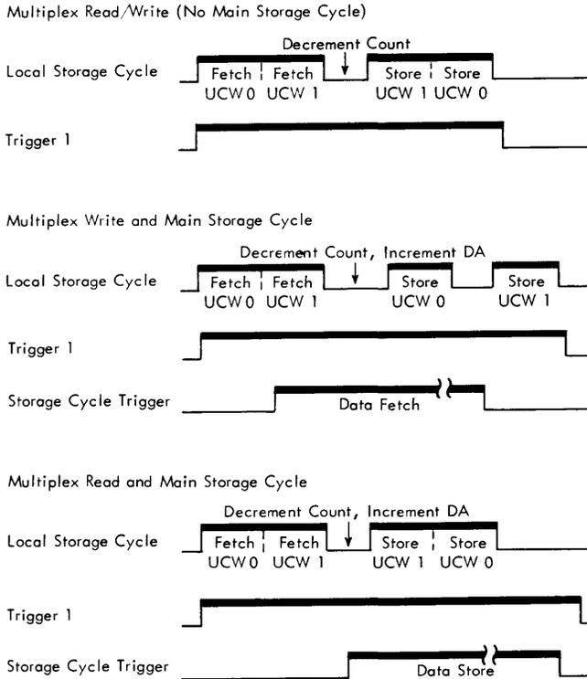
Figure 3-5. Multiplex Trigger 1
