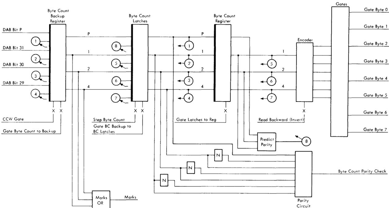
Figure 2-27. Selector Subchannel Byte Counter (Sheet 1 of 2)
