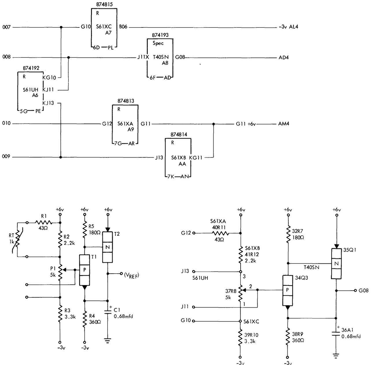
Figure B-1. Reference Voltage ( $V_{ref}$ )
