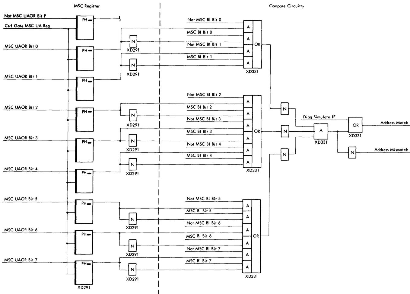
Figure 2-20. MSC Unit Address Register and Compare Circuits
