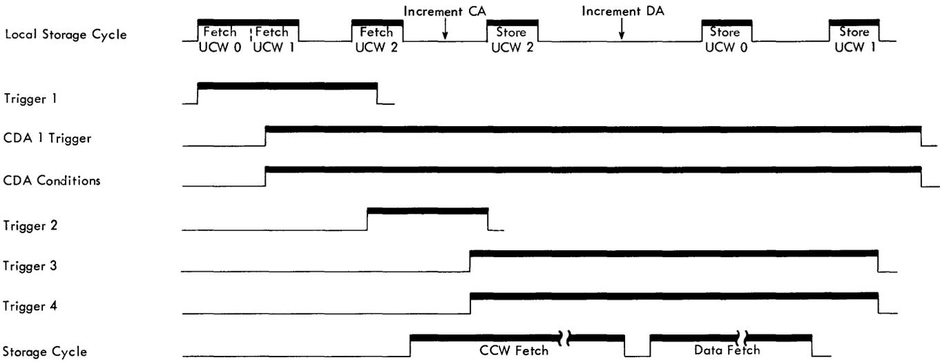
Figure 3-8. Multiplex CDA Trigger 1 (Prefetch Off)
