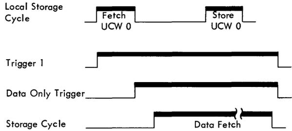
Figure 3-10. SSC Basic Trigger 1 and Data Only Trigger
