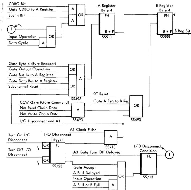
Figure 2-23. Selector Subchannel A and B Register Byte 4
