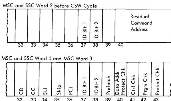
Figure 4-3. Unit Control Words with CPU ID Bits
