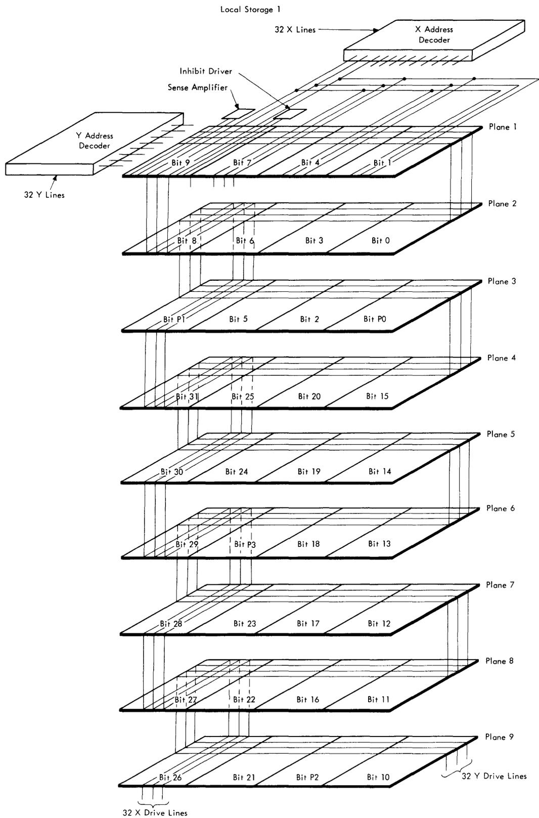
NOTE: There is an identical core array for local storage 2.
