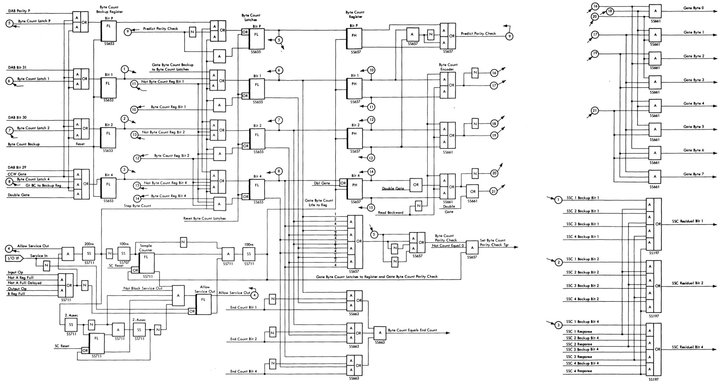
Figure 2-27. Selector Subchannel Byte Counter (Sheet 2 of 2)
