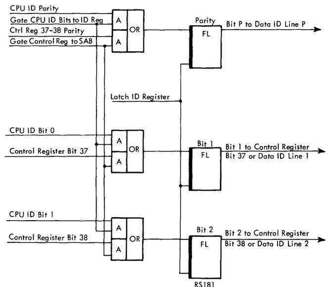
Figure 4-2. CPU Identity Register
