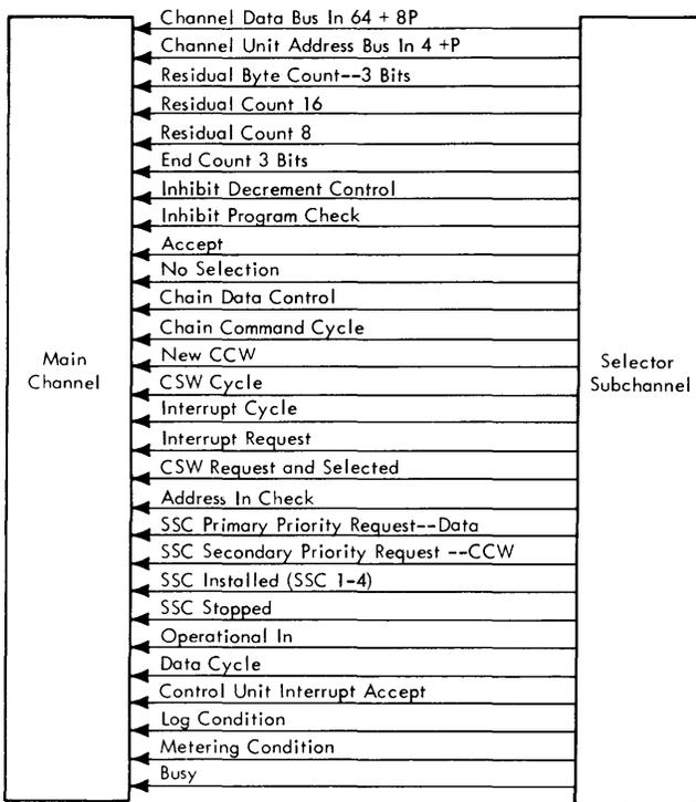
Figure 2-29. Selector Subchannel to Main Channel Interface
