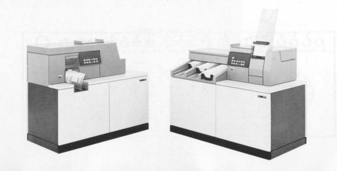
The photograph shows the 3525 Card Punch on the left, and the 3505 Card Reader on the right.
