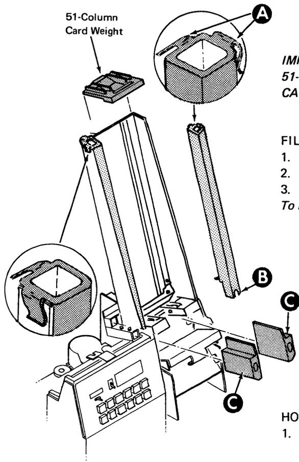
**IMPORTANT: ADAPTERS MUST BE INSTALLED TO PROCESS 51-COLUMN CARDS, AND REMOVED TO PROCESS 80-COLUMN CARDS.**
