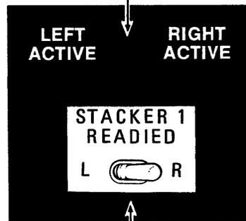
The readied toggle switch, which is set by the operator, indicates that a stacker is ready to receive cards after the active stacker becomes full.
