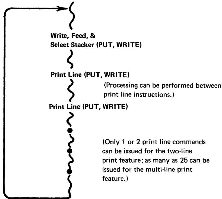
This file type (sequence of commands) should be used for punching and printing on blank cards because the command sequence allows the automatic subsystem punch retry function to occur in case of punching errors.
