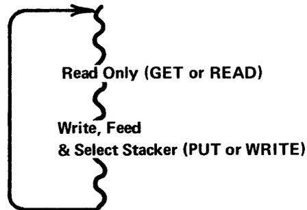
**Punching into Prepunched Cards:** This file type (that is, sequence of commands) should be used whenever you are punching data into prepunched cards, because the read-punch command sequence causes the subsystem to suppress the punch retry function for punching errors. If the punch retry function were not suppressed, and if a punch error were to occur, the subsystem would automatically try to punch data correctly into the following two cards.
