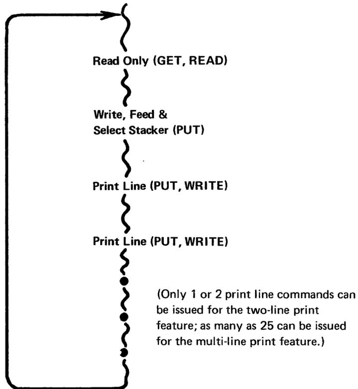
**Punching and Printing On Card That Is Being Read:** This file type (sequence of commands) should be used whenever prepunched cards are to be punched and printed: the read-punch command sequence causes the subsystem to suppress the punch retry function for mispunched cards. If the punch retry function were not suppressed, and if a punching error were to occur, the subsystem would try to repunch the data correctly into the following two cards.
