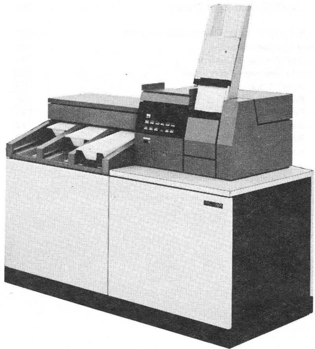
**IBM 3525 CARD PUNCH WITH AN IBM 3504 OR 3505 CARD READER**
