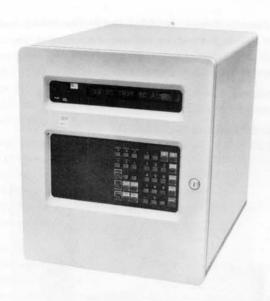
3644 Automatic Data Unit - A Programmable terminal, packaged for industrial environments, that provides the capability of attaching a variety of sensors, actuators, production, and laboratory equipment to the 3631/3632 controller. The highlights of the 3644 are:
