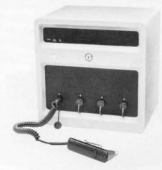
3646 Scanner Control Unit - A terminal packaged for industrial environments that allows attaching two Magnetic Hand Scanners or Magnetic Slot Readers. An optional feature allows attachement of two additional magnetic readers.
