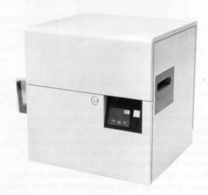
3643 Keyboard Display - The Models 2,3 and 4 provide 240, 480, and 1024 positions of display capability with either a seventy-four or ninety-four key alphanumeric keyboard. Additionally, a Magnetic Reader Attachment feature allows the Magnetic Hand Scanner or Magnetic Slot Reader to be attached.
