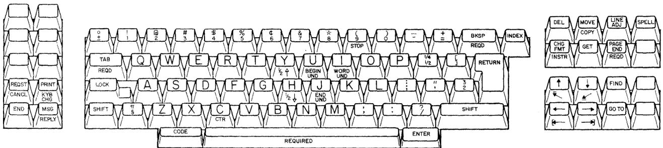
Figure 2-3. IBM Displaywriter System Keyboard
