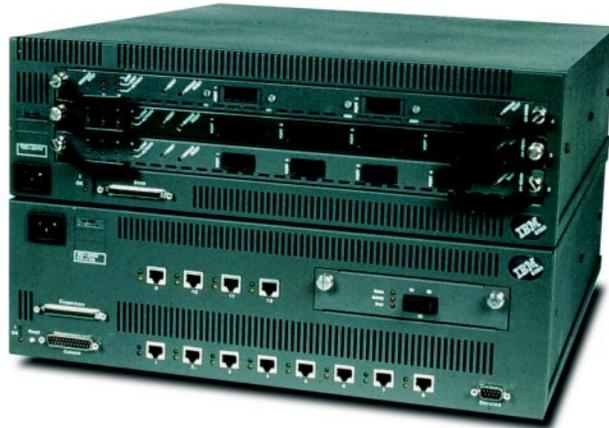
The IBM 8285 Nways<sup>®</sup> ATM Workgroup Switch is a multipurpose, expandable ATM switch that simplifies ATM implementation. It has twelve 25-Mbps ATM ports for desktop or server connections and a feature slot for optional 155-Mbps I/O cards for connecting to a server or another switch. I/O cards for 155-Mbps ATM on multimode fiber (MMF) and single-mode fiber (SMF) are supported.
