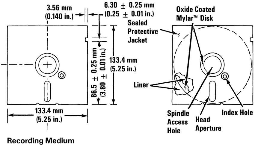
To load a diskette, the operator twists the latch at the front of the diskette drive counter-clockwise and inserts the diskette into the slot. Plastic guides in the slot ensure the diskette is in the correct position. Twisting the latch clockwise centers the diskette and clamps it to the drive hub. After 250 milliseconds, the servo-controlled dc motor starts and drives the hub at a constant speed of 300 rpm.
