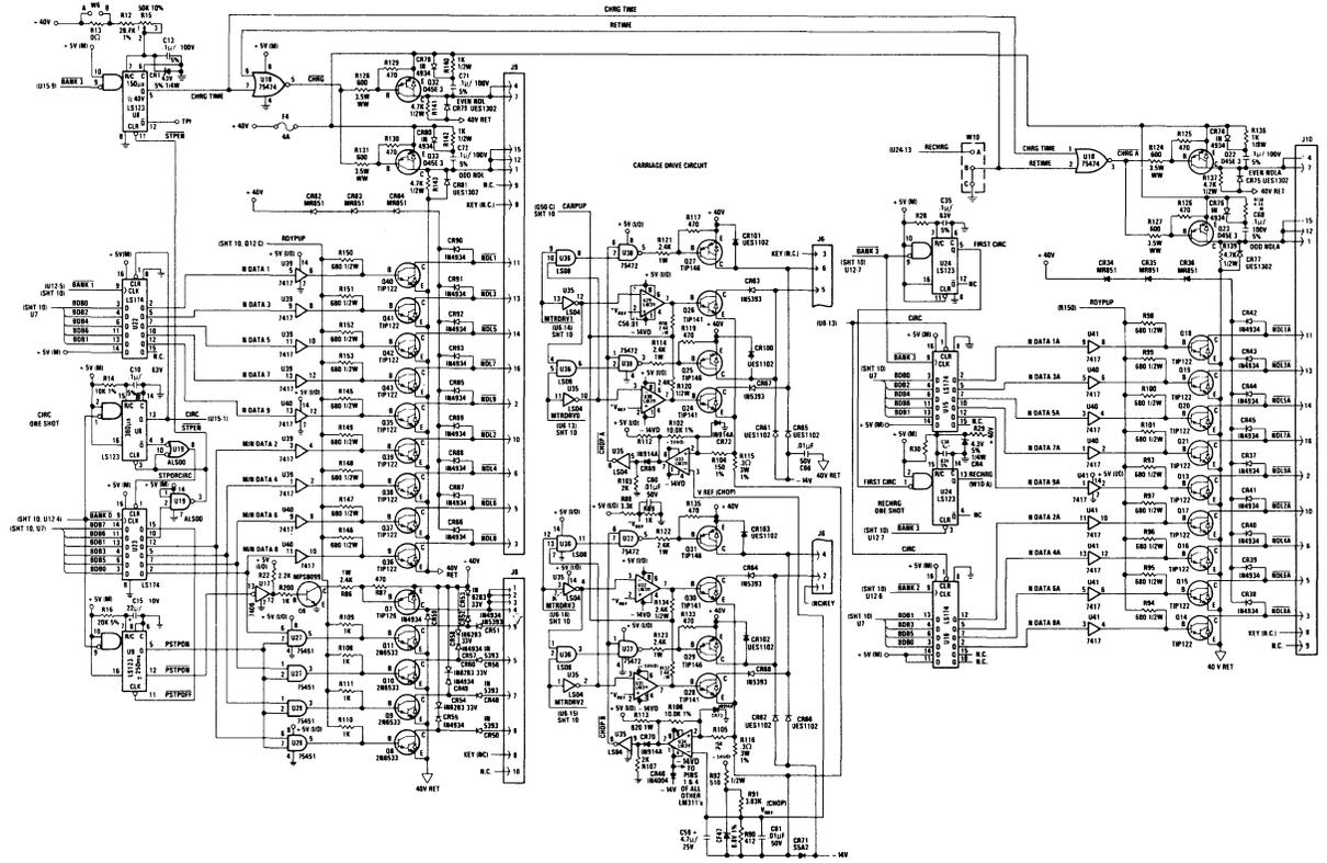
Color Printer — Controller Board (Sheet 2 of 3)
