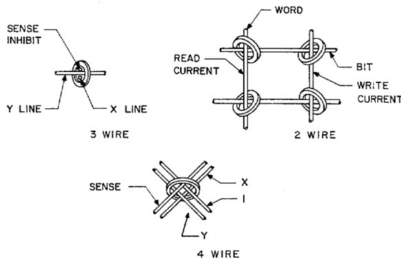
Fig. 1. Wire orientation.
