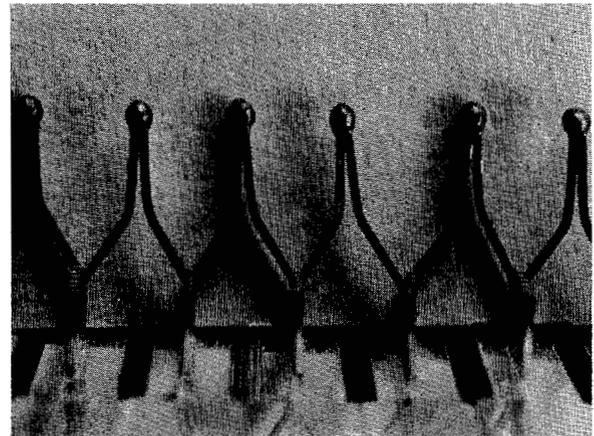
Fig. 25. EB and TIG typical welded terminals.
