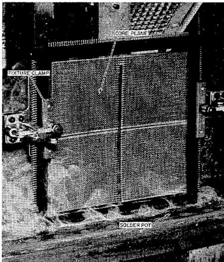
Fig. 15. Gang soldering.
