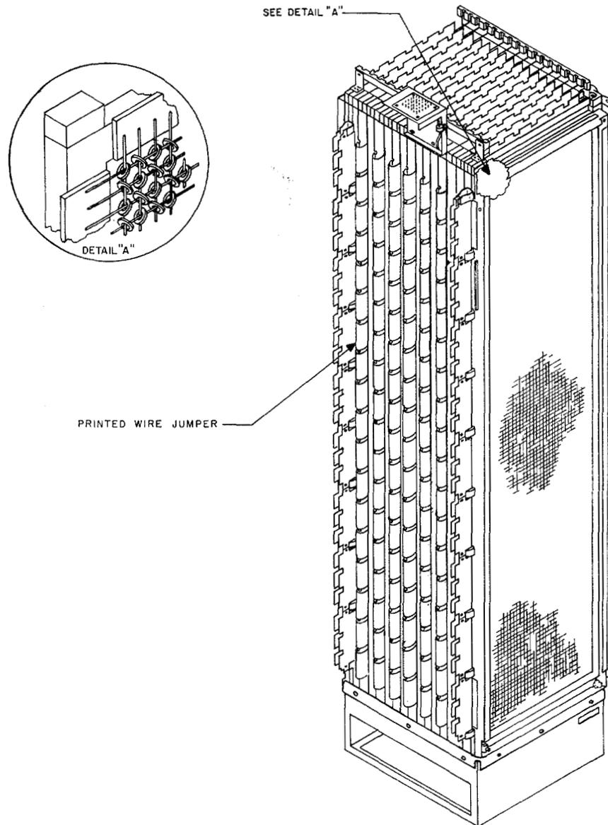
Fig. 20. Large capacity store array.
