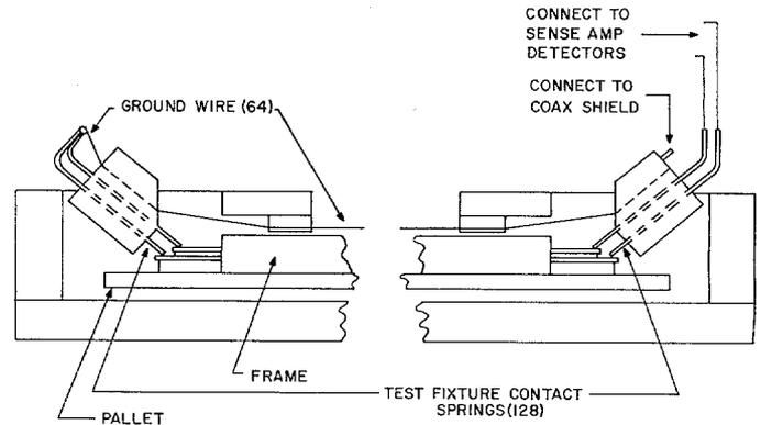
Fig. 10. Test fixture.
