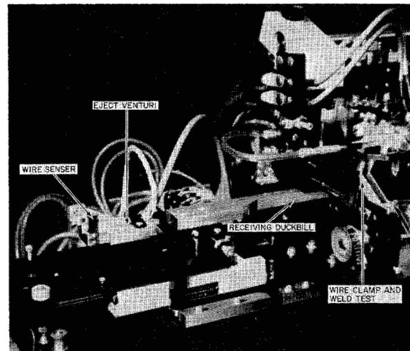
Fig. 14. Receiving mechanism.
