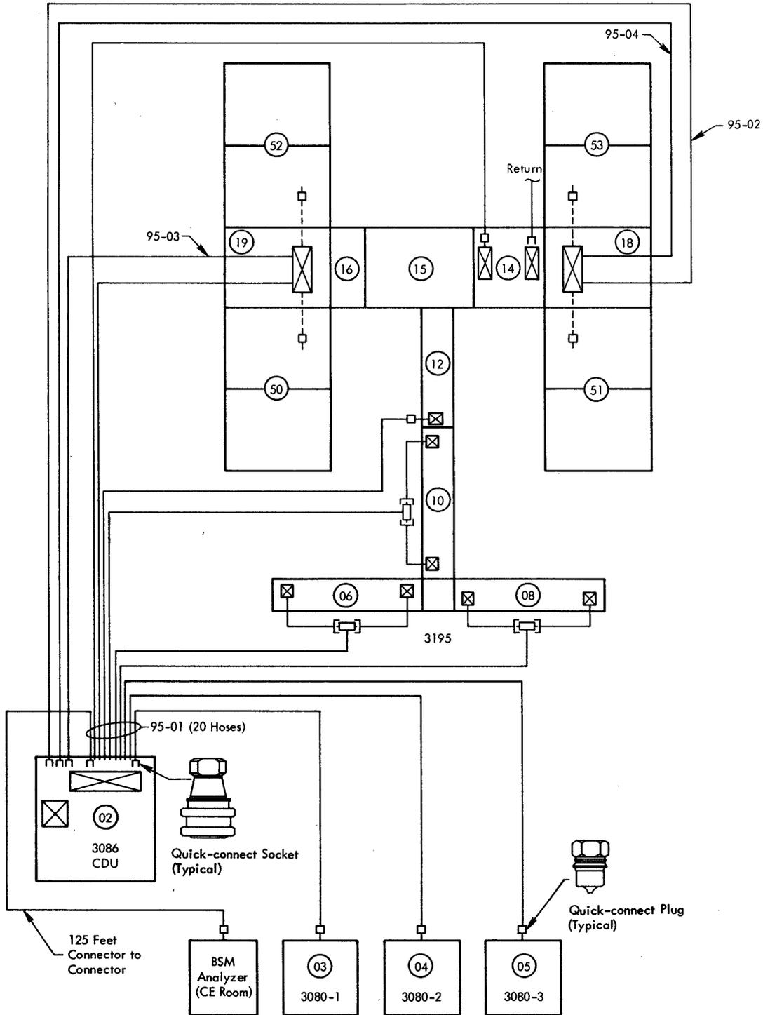
**SYSTEM/360 MODEL 195 CABLING SCHEMATIC—COOLANT HOSES**
