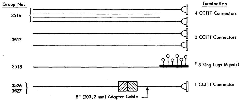
**SYSTEM/360 MODEL 25 CABLING SCHEMATIC (U.S.)**
