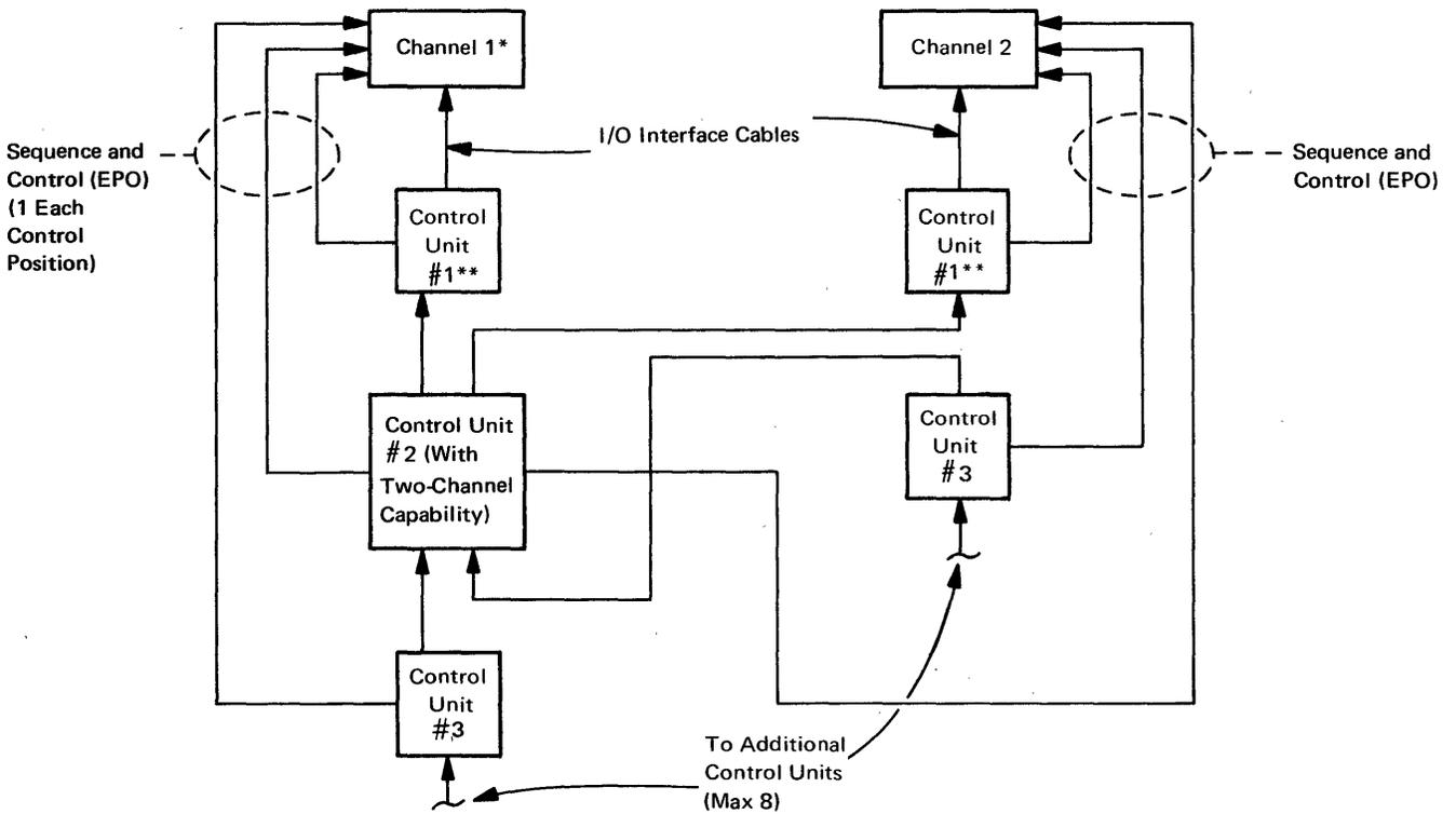
\*The channel may be a separate unit (such as the IBM 2860) or integral to the system processing unit.
