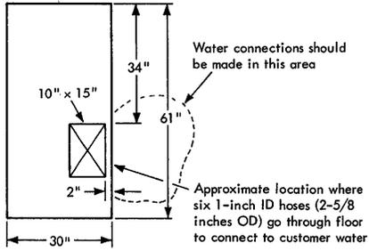
**Typical Connections for Customer-supplied Chilled Water
