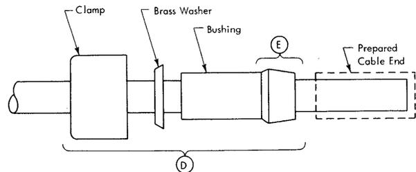
Slide the brass washer over the shield and up against the mating surface of the bushing at (F). Wrap tape around the shield for one full turn and trim off the remaining shield strands. Install the clamp and be sure that the mating surface is tightly against the brass washer.
