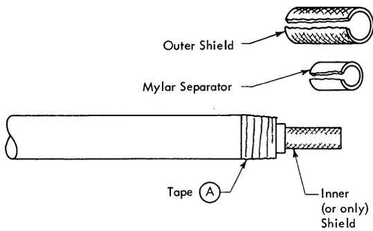
**Step 3:** (For two-shield cables only.) Remove Mylar separator for 1 inch (25 mm) from end for 15A-30A cables or 2-1/4 inches (57 mm) from end for 45A-60A cables. Do not cut the inner shield.
