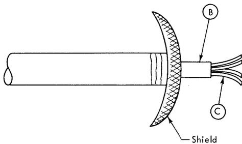
**Step 6:** Carefully lay the shield back over the cable outer jacket; wrap tape around the shield for temporary protec-
