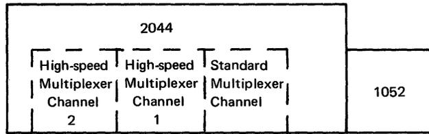
Up to eight control units per channel; maximum cable <sup>\*</sup> length per channel is 200 feet (unless modified by general control-to-channel cabling schematic)
