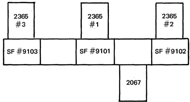
Example 14—SF #9103 attaches 2365 Model 2 #3 to 2067 Model 1 (2365 Model 2 with SF #9102 is a prerequisite).
