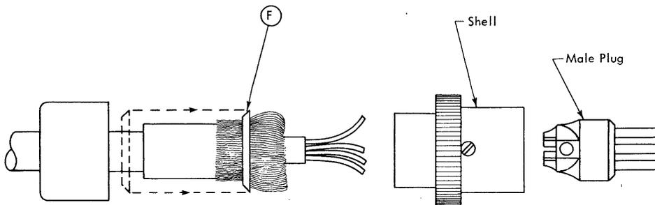
tion. Note that on two-shield cables, the outer shield must be insulated from the plug cap, equipment ground (earth) wire, conduit, and so on; the outer shield is grounded at the machine end only. The inner (or only) shield should be grounded through the shell of the plug to the branch circuit conduit. Three-hundred-sixty-degree grounding of the shield to the plug shell is desirable; that is, making contact between the shield and the shell at all points around the edge, not just at one point.
