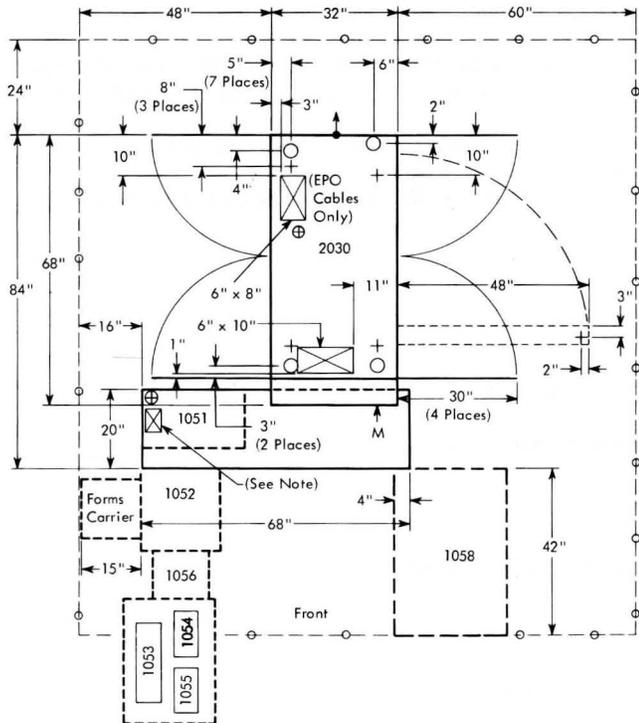
Note: This cable opening is required when SF # 3622 or 1051 is installed.
